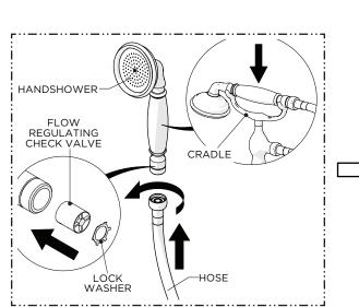
4. Thread the HOSE onto the HANDSHOWER and ensure it rests properly on the CRADLE.
