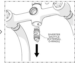
3. Remove the DIVERTER SHUTTLE from below.
