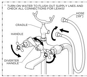
Thread the HOSE onto the CRADLE then turn on the water to flush out the supply lines and check all connections for leaks.
