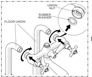
Using the RUBBER WASHERS provided, hold the TUB FILLER up to the UNIONS then thread and securely tighten the UNION NUTS onto the UNIONS.
