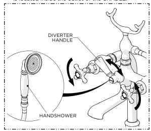
With water running, operate the DIVERTER HANDLE to ensure the HANDSHOWER functions properly.
