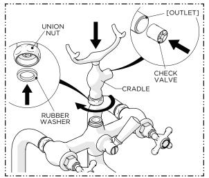
Using the RUBBER WASHER provided, thread and securely tighten the HANDSHOWER CRADLE onto the TUB FILLER.
