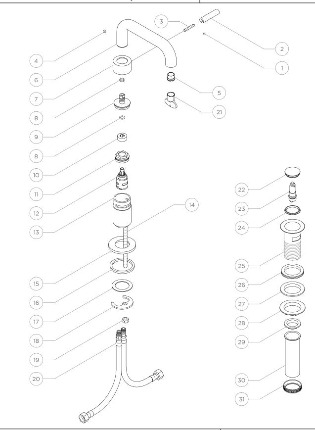
These guidelines have been prepared for the professional contractor to aid in the installation of: FLYTE LOW PROFILE ONE HOLE DECK MOUNTED LAVATORY FAUCET WITH METAL LEVER HANDLE (STYLE No. 417633).
