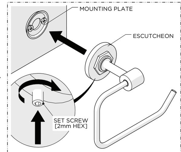
4. Place the product over the MOUNTING PLATE and securely tighten the SET SCREW.
