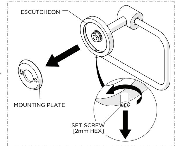
2. Loosen, but do **NOT** remove, the SET SCREW on the bottom of ESCUTCHEON using a 2mm HEX KEY and remove the MOUNTING PLATE.
