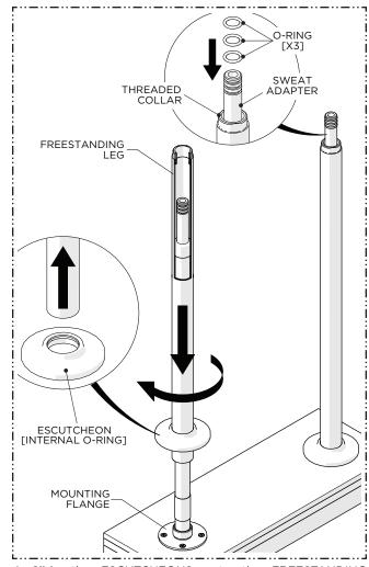
4. Slide the ESCUTCHEONS onto the FREESTANDING LEGS then slide the LEGS over the SUPPLY LINES and thread them onto the MOUNTING PLATES. Re-attach the O-RINGS onto the SWEAT ADAPTERS.
