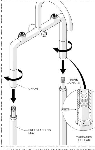
Slide the UNIONS onto the ADAPTERS and thread them onto the LEGS.
