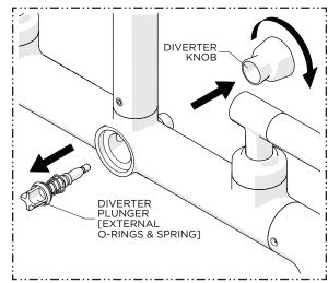
3. While holding the DIVERTER PLUNGER, unthread the KNOB from the PLUNGER then remove both
