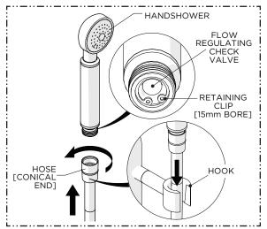
11. Thread the conical end of the HOSE to the HANDSHOWER then rest the HANDSHOWER on the HOOK.
