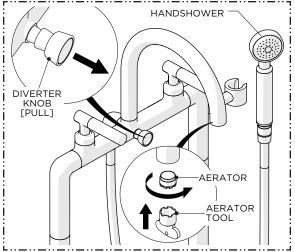
13. With water running, operate the DIVERTER KNOB to ensure it and the HANDSHOWER function properly then turn off the water and re-install the AERATOR.
