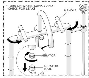
12. Remove the AERATOR using the TOOL provided then turn on the water supply and operate the HANDLES to flush out the supply lines and check all connections for leaks.
