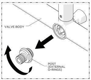
2. Unthread and remove the POST from the VALVE BODY.
