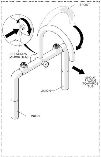
5. Align the SPOUT properly and securely tighten the SET SCREW at the base of the SPOUT.
