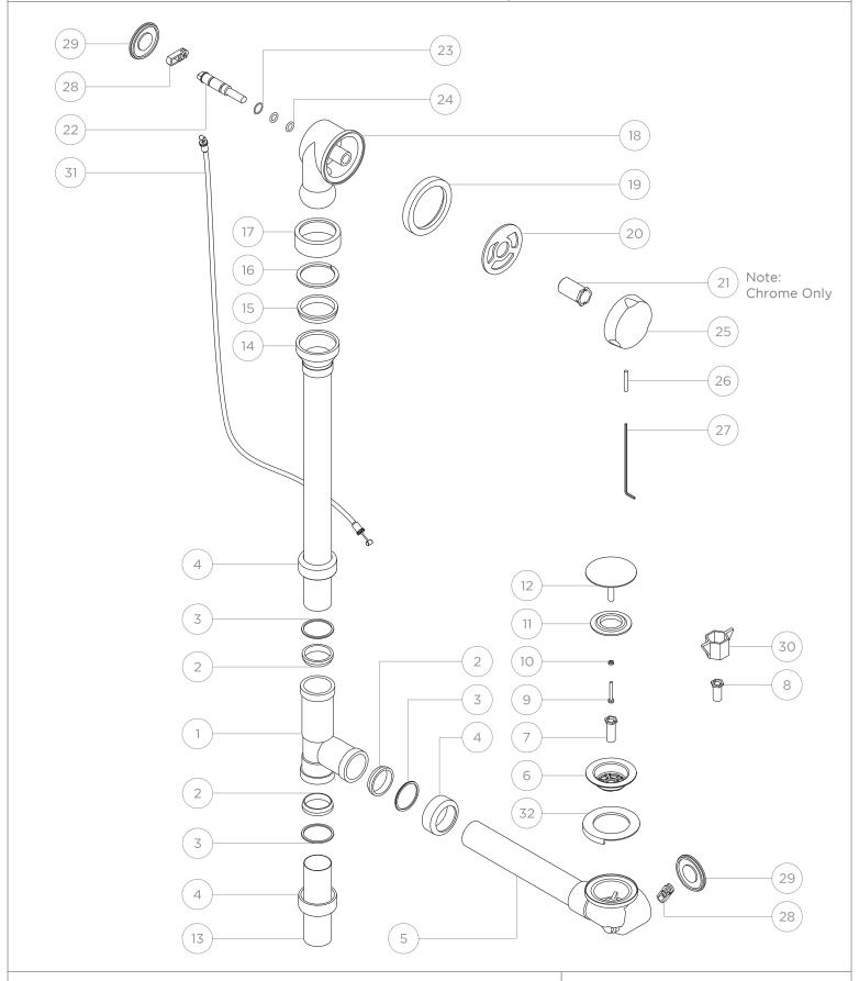
These guidelines have been prepared for the professional contractor to aid in the installation of: <a href="UNIVERSAL POP-UP WASTE AND OVERFLOW DRAIN">UNIVERSAL POP-UP WASTE AND OVERFLOW DRAIN (STYLE No. UNWO51)</a>.
