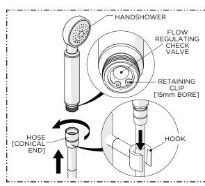
9. Thread the conical end of the HOSE to the HANDSHOWER then rest the HANDSHOWER on the HOOK.
