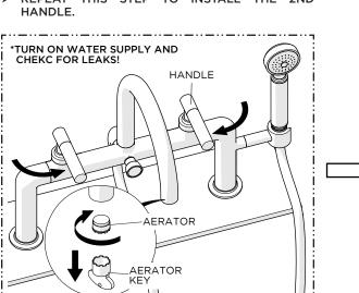
10. Remove the AERATOR using the TOOL provided then turn on the water supply and operate the HANDLES to flush out the SUPPLY LINES and check all connections for leaks.
