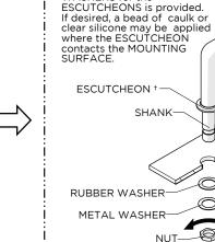
2. Insert the SHANKS into the holes on the MOUNTING SURFACE then attach the RUBBER and METAL WASHERS and NUTS onto the SHANKS. Securely tighten the NUTS against the underside of the MOUNTING SURFACE.
