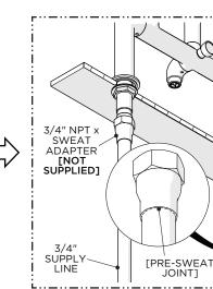
3. Pre-sweat 3/4" female NPT x SWEAT ADAPTERS to 3/4" SUPPLY LINES and let cool. Apply a thin coat of pipe thread sealant to the male threads on the SHANKS then thread and securely tighten the ADAPTERS onto the SHANKS.
