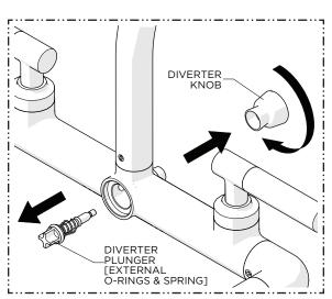
While holding the DIVERTER PLUNGER, unthread the KNOB from the PLUNGER then remove both parts.
