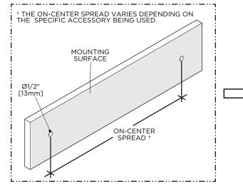
1. Ensure any pre-drilled hole is a 1/2" [13mm]. For ACCESSORIES with 2 mounting holes, ensure the holes are level and at the proper on-center spread.
