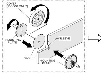
Insert the SLEEVE into the pre-drilled hole, insert the SET SCREW through the SLEEVE, and slide the second GASKET onto the SCREW then thread the COVER, or second MOUNTING PLATE, onto the SCREW.
