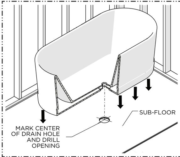
1. Determine the placement of the BATHTUB and mark the location of the drain hole then drill a hole through the floor to accommodate the DRAIN (SOLD SEPARATELY).
