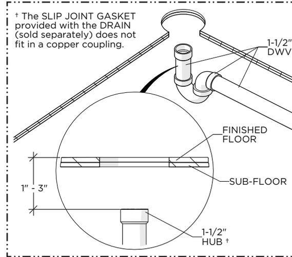
2. Rough-in a 1-1/2" DWV (not supplied). The top of the HUB must be 1"- 3" from the finished floor in order for the TAILPIECE to be securely installed. Ensure all DWV pipes and fittings are well supported to eliminate the possibility of shifting.
