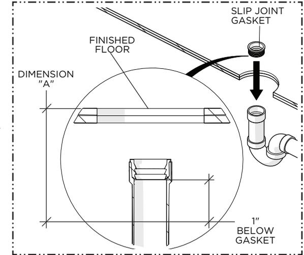
3. Insert the SLIP JOINT GASKET into the HUB then measure from the finished floor to 1" [25mm] past the bottom of the GASKET.
