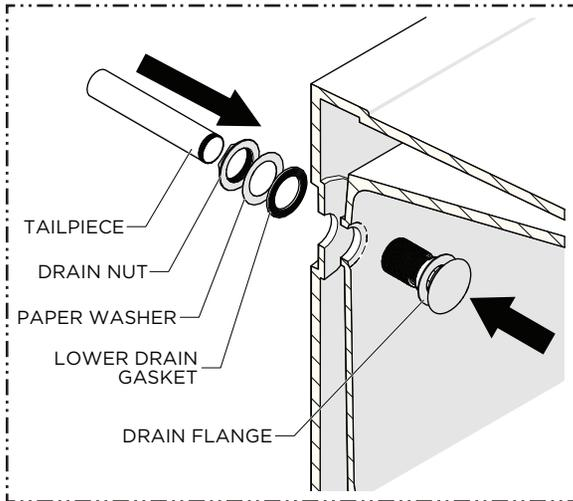
4. Cover the floor with a pad or other protective material and gently rest the BATHTUB on its side then dry-fit the DRAIN (UNWO15 is shown - SOLD SEPARATELY).
