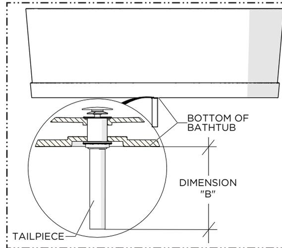
5. Measure the distance the TAILPIECE protrudes past the bottom of the BATHTUB.
