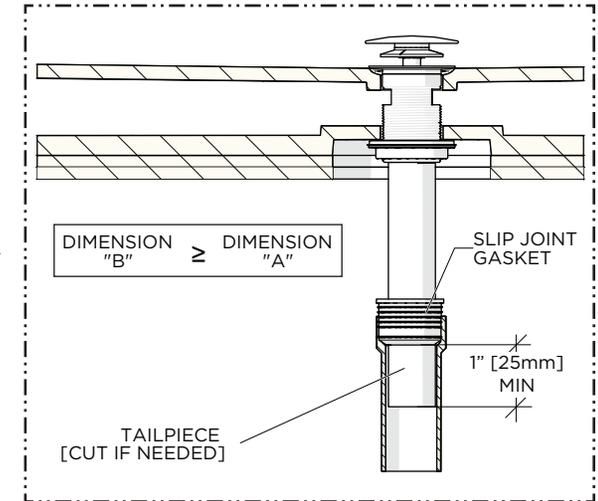
6. **IMPORTANT:** Verify DIMENSION B is greater than or equal to DIMENSION A. This will ensure that the TAILPIECE will extend a MINIMUM of 1" past the SLIP JOINT GASKET. If necessary, cut the TAILPIECE.
