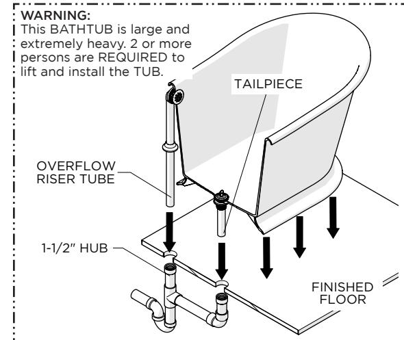
12. Position the BATHTUB and align the TAILPIECE and OVERFLOW RISER TUBE with the DRAIN HUBS then carefully lower the BATHTUB until it rests on the finished floor.
