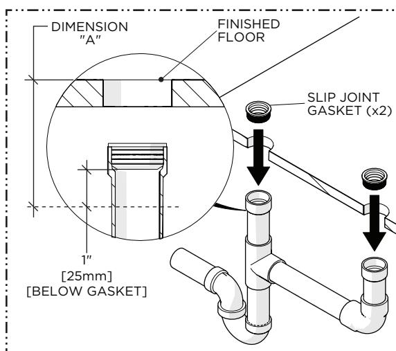
1. Insert the SLIP JOINT GASKETS (x2) into the HUBS then measure from the finished floor to 1" [25mm] below the bottom of the GASKETS.
