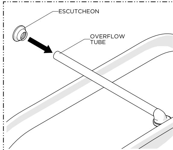
10. Slide the ESCUTCHEON onto the OVERFLOW RISER TUBE.
