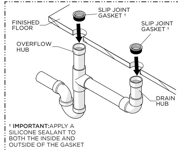
11. Apply a generous coating of a clear adhesive silicone sealant to both the inside and outside of the SLIP JOINT GASKETS and insert the GASKETS into the DRAIN HUBS.
