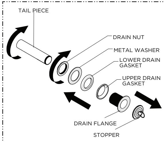
4. Remove the STOPPER, UPPER and LOWER DRAIN GASKETS, WASHERS, NUT and TAILPIECE from the DRAIN FLANGE.
