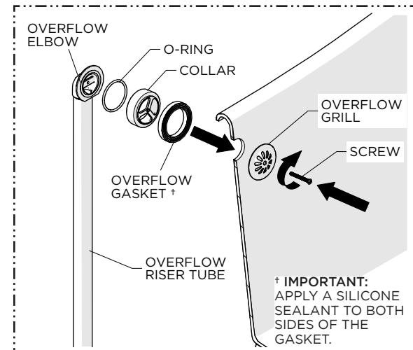
9. Apply a generous bead of silicone sealant to both sides of the OVERFLOW GASKET then assemble the OVERFLOW RISER TUBE to the BATHTUB making sure to include the COLLAR and O-RING and securely tightening the SCREW.
