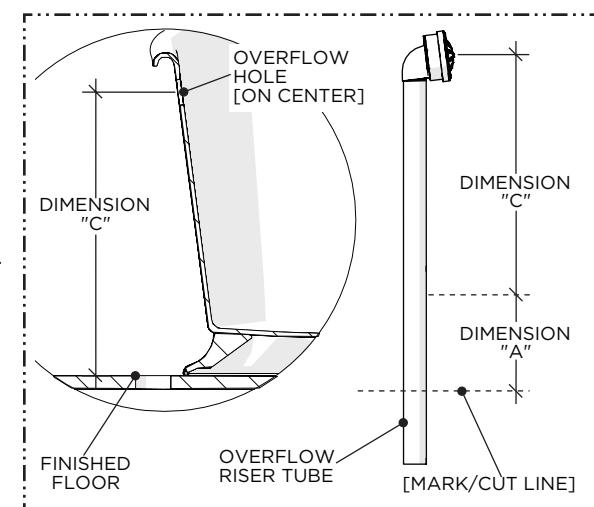
3. Measure (DIMENSION "C") from the center of the OVERFLOW HOLE to the finished floor then, using the previous DIMENSION "A", mark and cut the OVERFLOW RISER TUBE.
