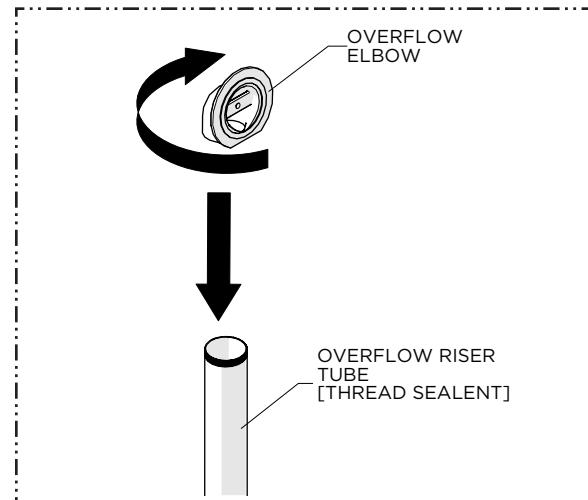
8. Apply thread sealant or pipe dope to the threads on the RISER TUBE then thread and securely tighten the ELBOW onto the TUBE.
