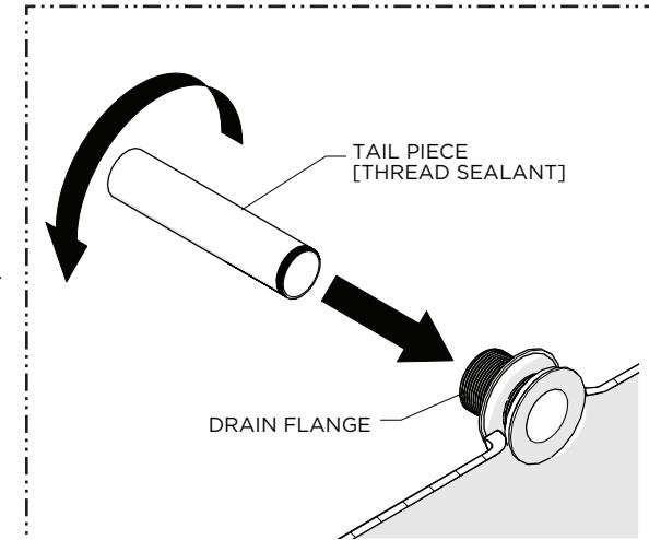
6. Thread the TAILPIECE into the DRAIN FLANGE.
