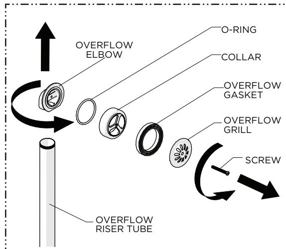
7. Unthread and remove the SCREW, OVERFLOW GRILL, OVERFLOW GASKET, COLLAR, and ORING. Remove OVERFLOW RISER PIPE from OVERFLOW ELBOW.
