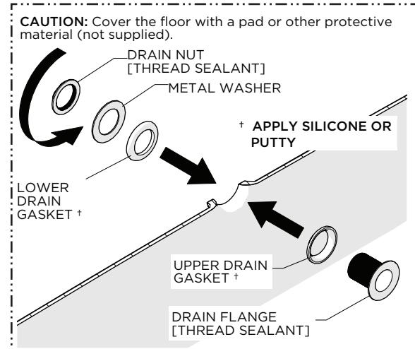
5. With the BATHTUB on its side, apply a generous bead of silicone or putty to the UPPER and LOWER GASKETS and set the FLANGE then thread and securely tighten the NUT onto the FLANGE.
