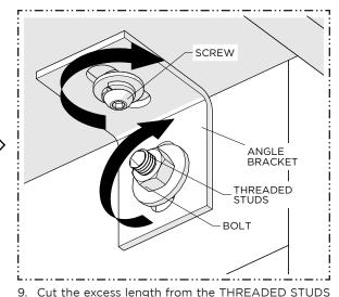
then securely and evenly tighten the NUTS and SCREWS to secure the ANGLE BRACKETS.
