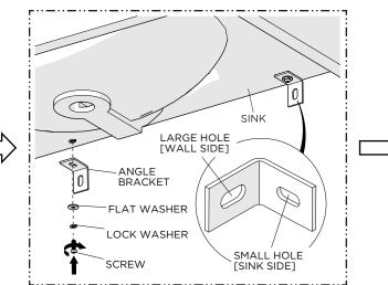
5. Install the ANGLE BRACKET to the underside of the SINK using the SCREWS and WASHERS PROVIDED. Do **NOT** tighten the SCREWS.
