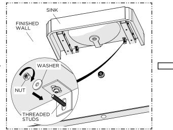
8. Place the SINK on top of the BRACKETS and push it against the FINISHED WALL. Install the WASHERS and NUTS provided onto the THREADED STUDS and hand-tighten.
