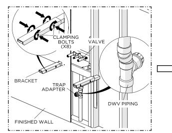
4. Once the level is set, tighten the CLAMPING BOLTS on both BRACKETS to secure the level. Ensure the PLUMBING SUPPLY and TRAP ADAPTER are properly installed before completing the FINISHED WALL installation.
