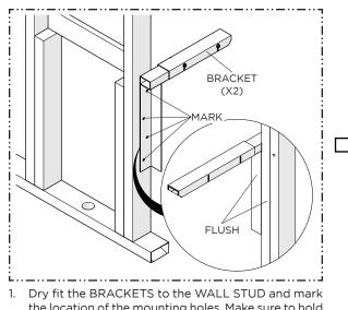
Dry fit the BRACKETS to the WALL STUD and mark the location of the mounting holes. Make sure to hold the BRACKETS level and flush with the front face of the STUD. Drill pilot holes for the 3/8" [10mm] LAG SCREWS provided.
