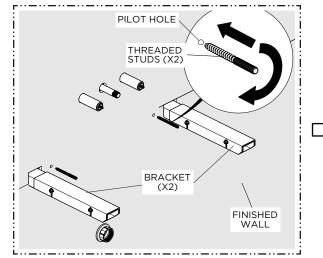
7. Install the M8 THREADED STUDS making sure the wood end is fully inserted into the FINISHED WALL, then apply adhesive silicone to the top surfaces of the SUPPORT BRACKETS.
