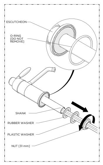
† An O-RING for the **ESCUTCHEON** is **HANDLE** provided. If desired, a bead of caulk or clear silicone may be applied where the **ESCUTCHEON** contacts the mounting surface. ESCUTCHEON † **SPOUT** TOWARDS SINK SHANK-**MOUNTING** SURFACE RUBBER WASHER INLET/OUTLET **TUBES** PLASTIC WASHER NUT [31 mm]
