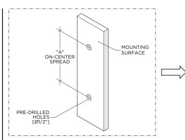
1. Drill two 1/2" diameter holes on the mounting surface at the required on-center spread (DIM A).
