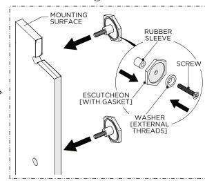
2. Pre-assemble the WASHERS, ESCUTCHEONS, and RUBBER SLEEVES onto the SCREWS then insert the RUBBER SLEEVES into the pre-drilled holes.
