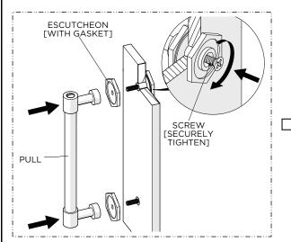
3. Slide the ESCUTCHEONS onto the SCREWS and align the holes on the PULL then thread and securely tighten the SCREWS into the PULL.
