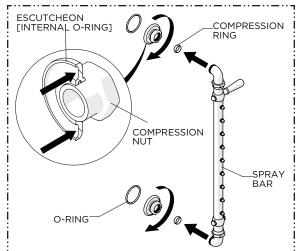
Slide the ESCUTCHEONS up the COMPRESSION NUTS then unthread and remove the NUTS from the SPRAY BAR.
