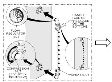
4. Slide the BAR over the SUPPLIES then thread and securely tighten the COMPRESSION NUTS onto the BAR. The SPRAY BAR can be installed with the HANDLE on the top or bottom.
