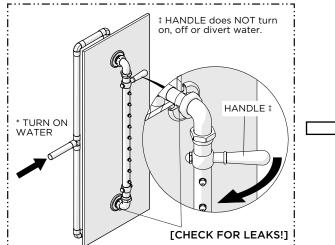
5. Turn on the water and a diverter/wall valve (sold separately), operate the HANDLE to ensure it functions properly, and inspect all connections for leaks then turn the water off
