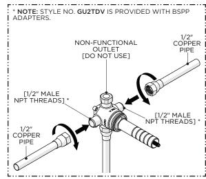
3. Run 1/2" copper supply lines from the outlet ports to the 2 desired devices making sure all piping and fittings are secured.
