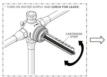
Turn on the water supply and operate the CARTRIDGE STEM to flush out the lines and check for leaks.
