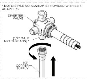
From the THERMOSTATIC VALVE being used, run a copper supply line to the proper height of the DIVERTER VALVE making sure it's positioned according to the VALVE MARKINGS so that mixed water flows into the inlet and all piping and fittings are secured
