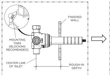
The VALVE rough-in depth is measured from the center of the inlets to the surface of the finished wall and VARIES depending on the TRIM used.
