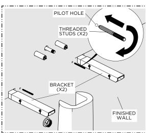
Install the M8 THREADED STUDS making sure the wood end is fully inserted into the FINISHED WALL, then apply adhesive silicone to the top surfaces of the SUPPORT BRACKETS.
