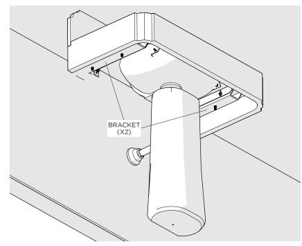
**NOTE:** The SINK will be supported by the brackets and not the PEDESTAL. Ensure the SINK is not resting on the PEDESTAL to avoid damage.
