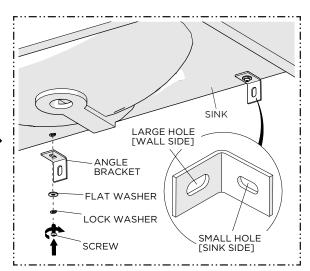
Install the ANGLE BRACKET to the underside of the SINK using the SCREWS and WASHERS PROVIDED. Do NOT tighten the SCREWS.
