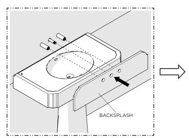
10. Install the BACKSPLASH provided using an adhesive silicone.
