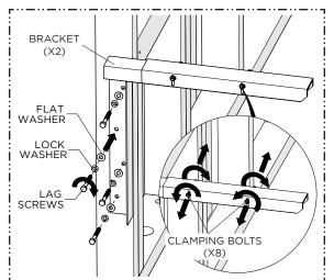
Install both BRACKETS with the provided LAG SCREWS and WASHERS, ensuring they are securely attached, Once installed, loosen the CLAMPING BOLTS on each bracket, but do not remove them.
