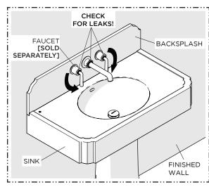
12. Turn on the water and operate the drain and FAUCET [sold separately] to ensure proper operation. Check all connections for leaks. If desired, a bead of caulk or clear silicone may be applied where the SINK contacts the FINISHED WALL.
