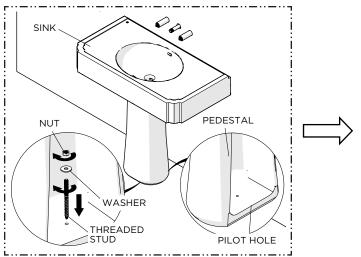
Dry fit the PEDESTAL to fit in front of the drain hole of the SINK. Mark where the hole is, drill, and secure the position using THREADED STUD, WASHER, and NUT.
