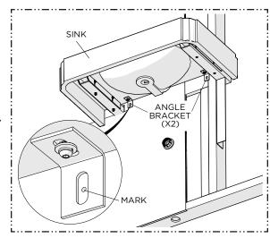
Dry fit the SINK with SUPPORT BRACKETS ensuring it is level. Mark the hole locations for the ANGLE BRACKETS then remove the SINK and drill pilot holes for M8 THREADED STUDS.
