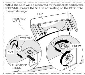
Place the SINK on BRACKETS against the FINISHED WALL. Install WASHERS and NUTS on THREADED STUDS and hand-tighten. Cut excess from STUDS, then securely tighten NUTS and SCREWS on ANGLE BRACKETS.
