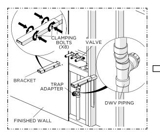
Once the level is set, tighten the CLAMPING BOLTS on both BRACKETS to secure the level. Ensure the PLUMBING SUPPLY and TRAP ADAPTER are properly installed before completing the FINISHED WALL installation.
