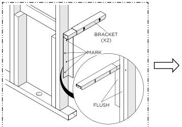
Dry fit the BRACKETS to the WALL STUD and mark the location of the mounting holes. Make sure to hold the BRACKETS level and flush with the front face of the STUD. Drill pilot holes for the 3/8" [10mm] LAG SCREWS provided.
