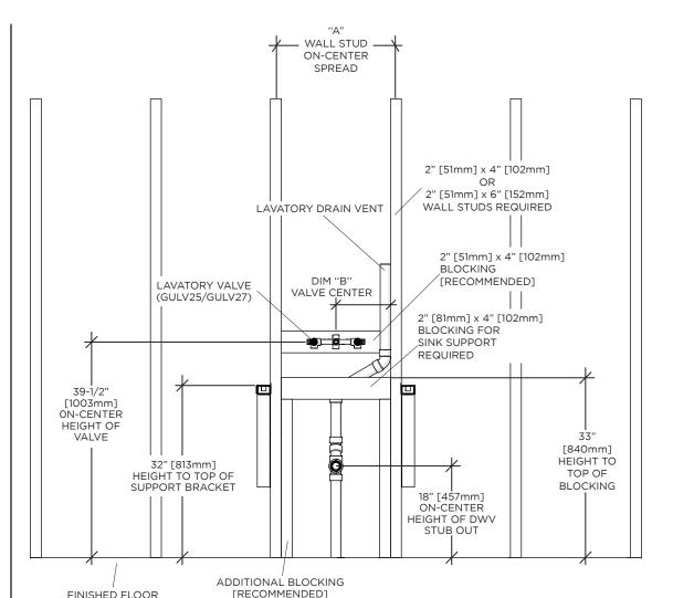
NOTE: This blocking scheme installs the sink top 34" [864mm] from the floor.
