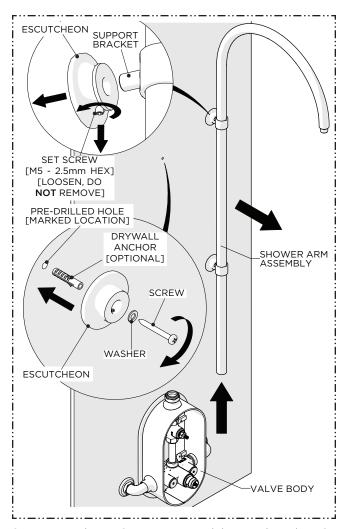
Remove the SHOWER ARM and loosen, but do NOT remove the SET SCREW on the bottom of the SUPPORT POST ESCUTCHEON. Using the previous marks, predrill a hole (pilot hole) to accommodate the MOUNTING SCREW and, if blocking is not installed, install the DRYWALL ANCHOR provided.
