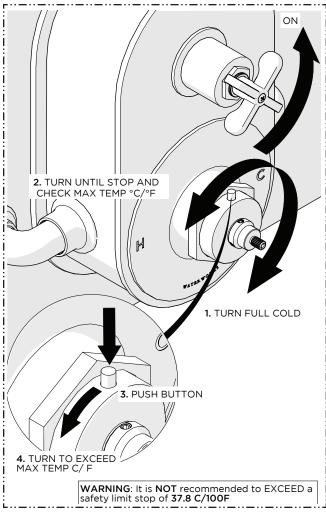
19. Turn the LIMIT STOP to cold then hot and confirm it is functioning properly. Verify the maximum desired bathing temperature. To get a hotter temperature, press and hold the LIMIT STOP BUTTON and turn the LIMIT STOP further.
