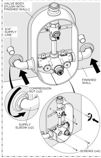
7. Fit the SUPPLY ELBOWS onto the SUPPLY LINES making sure the VALVE BODY sits flush against the finished wall and secure the VALVE BODY to the wall using the SCREWS (x4) provided then thread and securely tighten the COMPRESSION NUTS onto the ELBOWS.
