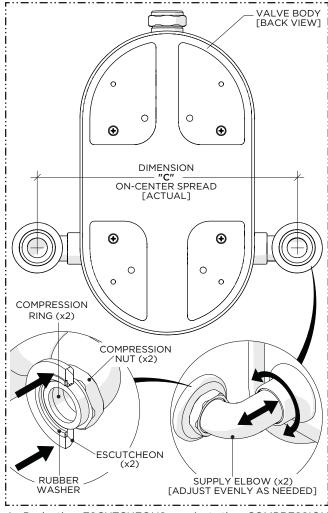
4. Push the ESCUTCHEONS against the COMPRESSION NUTS then measure the on-center spread of the SUPPLY ELBOWS (DIMENSION C).
