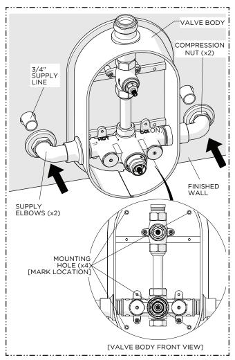
Dry-fit the SUPPLY ELBOWS onto the SUPPLY LINES making sure the VALVE BODY sits flush against the finished wall then mark the location of the MOUNTING HOLES (x4).
