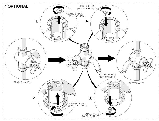
**NOTE:** The DIVERTER VALVE is set for a RIGHT HAND installation of the OUTLET ELBOW. If a LEFT HAND installation is desired, the LARGE and SMALL PLUGS must be swapped.
