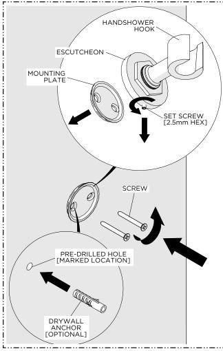
12. Loosen, but do NOT remove, the SET SCREW on the HANDSHOWER HOOK to remove the MOUNTING PLATE then determine the ideal and/or desired location for the HOOK and secure the MOUNTING PLATE using the SCREWS provided. If blocking is not installed, install the DRYWALL ANCHOR provided.
