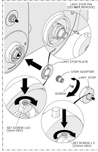
18. Place the LIMIT STOP PLATE onto the THERMOSTATIC VALVE in the desired orientation, securely tighten the SET SCREWS, place the STEM ADAPTER onto the CARTRIDGE then secure it using the SCREW provided.
