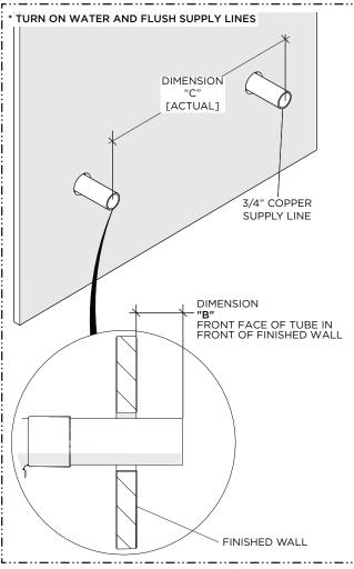
Measure the actual on-center spread (DIMENSION C) of the SUPPLY LINES, which MUST be between 11-1/8" [283mm] and 11-5/8" [295mm].
