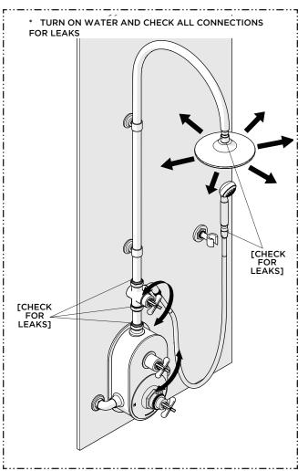
22. Turn on the water and operate the SHOWERHEAD to ensure it pivots and functions properly.
