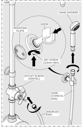
13. Place the HOOK onto the MOUNTING PLATE and securely tighten the SET SCREW then connect the HOSE to the HANDSHOWER and DIVERTER VALVE and place the HANDSHOWER on the HOOK.
