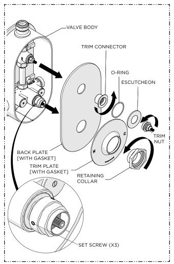
THERMOSTATIC HANDLE: Unthread and remove the RETAINING COLLAR then remove the TRIM PLATE.
