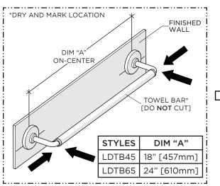
1. Dry-fit the TOWEL BAR to the finished wall and mark the ideal location making sure to hold the BAR level.
