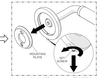
Loosen, but do NOT remove, the SET SCREW on the bottom of each ESCUTCHEONS and remove the MOUNTING PLATES.
