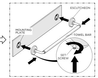
4. While holding the ENDS and BAR together, place the ESCUTCHEONS onto the MOUNTING PLATES making sure they are fully seated, securely tighten the SET SCREWS using 1/16" [1.5 mm] HEX key.
