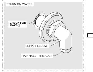
7. Turn on the water and a diverter/wall valve (sold separately) to flush out any debris in the supply line and inspect all connections for leaks then turn the water off.
