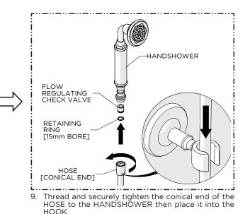
**NOTE:** A FLOW REGULATING CHECK VALVE is located in the inlet of the HANDSHOWER.
