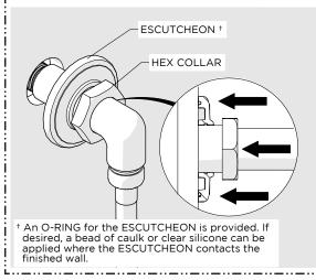
10. Slide the ESCUTCHEON and HEX COLLAR down the SUPPLY ELBOW until they contact the finished wall.
