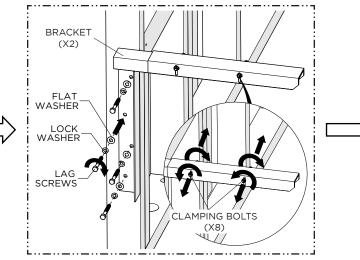
2. Install both BRACKETS with the provided LAG SCREWS and WASHERS, ensuring they are securely attached, Once installed, loosen the CLAMPING BOLTS on each bracket, but do **not** remove them.
