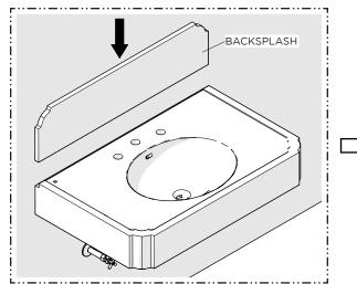
10. Install the BACKSPLASH provided using an adhesive silicone.
