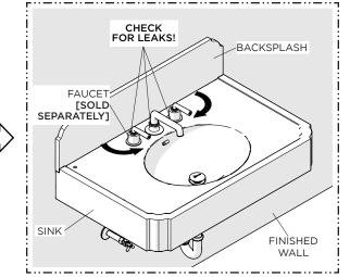
12. Turn on the water and operate the drain and FAUCET [sold separately] to ensure proper operation. Check all connections for leaks. If desired, a bead of caulk or clear silicone may be applied where the SINK contacts the FINISHED WALL.
