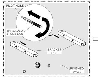
7. Install the M8 THREADED STUDS making sure the wood end is fully inserted into the FINISHED WALL, then apply adhesive silicone to the top surfaces of the SUPPORT BRACKETS.
