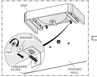
8. Place the SINK on top of the BRACKETS and push it against the FINISHED WALL. Install the WASHERS and NUTS provided onto the THREADED STUDS and hand-tighten.
