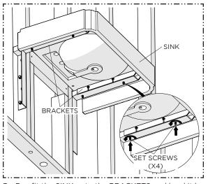
Dry-fit the SINK onto the BRACKETS and level it by adjusting the SET SCREWS at the bottom of each BRACKETS, Ensure the SINK'S weight is properly supported on the BRACKETS. Once aligned, remove the SINK and store it safely until the final installation.
