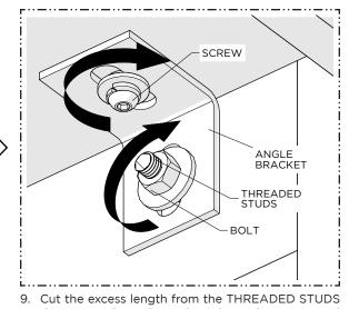
then securely and evenly tighten the NUTS and SCREWS to secure the ANGLE BRACKETS.
