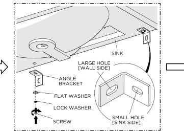
5. Install the ANGLE BRACKET to the underside of the SINK using the SCREWS and WASHERS PROVIDED. Do **NOT** tighten the SCREWS.
