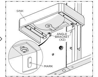
6. Dry fit the SINK with SUPPORT BRACKETS ensuring it is level. Mark the hole locations for the ANGLE BRACKETS then remove the SINK and drill pilot holes for M8 THREADED STUDS.
