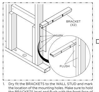
the location of the mounting holes. Make sure to hold the BRACKETS level and flush with the front face of the STUD. Drill pilot holes for the 3/8" [10mm] LAG SCREWS provided.
