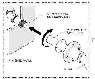
Making sure the NIPPLE (not supplied) is properly roughed-in, thread and securely tighten the SPOUT onto the NIPPLE.
