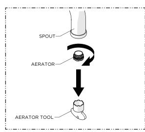
3. Using the TOOL provided, remove the AERATOR.
