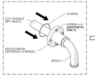
Slide the ESCUTCHEON and O-RING onto the SPOUT.
