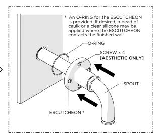
Slide the ESCUTCHEON down the SPOUT until it contacts the finished wall.
