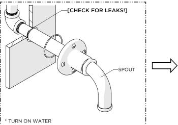
4. Turn on the water and a diverter/wall valve (sold separately) to flush out any debris in the supply line and inspect all connections for leaks then turn the water off.
