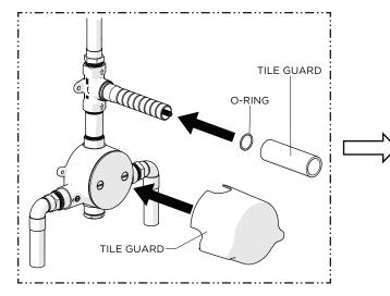
7. Place both TILE GUARDS onto the VALVE making sure they are FULLY seated.
