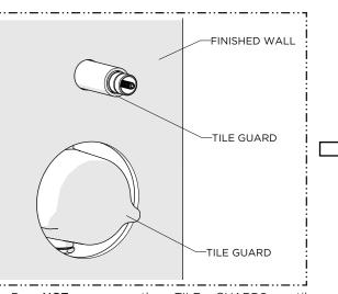
8. Do **NOT** remove the TILE GUARDS until construction is completed.
