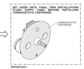
9. SET ASIDE THE THERMOSTATIC CARTRIDGE UNTIL FINAL TRIM INSTALLATION MAKING SURE TO REPEAT THE FLUSHING PROCESS AS NEEDED BEFORE INSTALLING THE CARTRIDGE.
