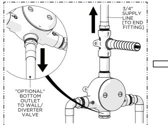
4. Run a 3/4" supply line from the top outlet to the desired end fitting (sold separately) making sure to secure all piping and fittings.
