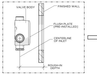
See the Installation Guidelines of the specific TRIM (sold separately) being used for the MAX and MIN rough-in depth dimensions.
