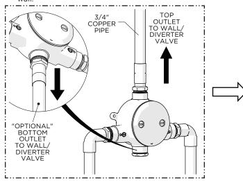
4. Run a 3/4" copper line from the top outlet and bottom outlet, if used, to a diverter/wall valve (sold separately) making sure to secure all piping and fittinas.
