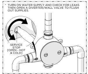
Turn on the water supplies then open the SERVICE STOPS (hot & cold) and open a diverter/wall valve to flush out the lines and check for leaks.
