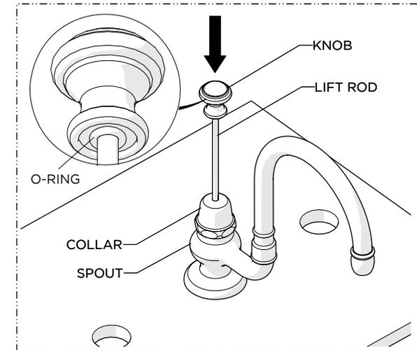
6. Insert the LIFT ROD into the top of the SPOUT making sure the O-RING is beneath the KNOB.
