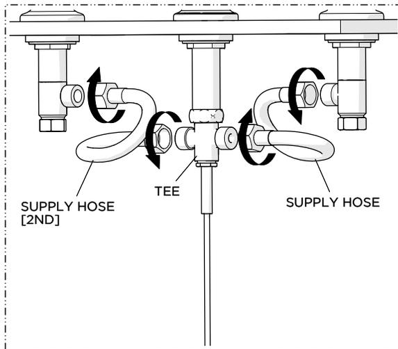
14. Connect the SIDEBODIES to the TEE using the SUPPLY HOSES and RUBBER WASHER provided. Securely tighten the HOSES and ensure they are not pinched/kinked.
