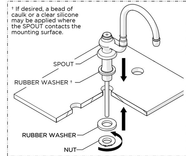
3. Insert the SHANK through the hole on the mounting surface making sure the RUBBER WASHER provided is beneath the SPOUT then re-attach the lower deck WASHER and securely tighten the NUT.
