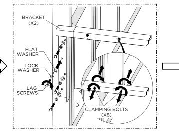
2. Install both BRACKETS with the provided LAG SCREWS and WASHERS, ensuring they are securely attached, Once installed, loosen the CLAMPING BOLTS on each bracket, but do **not** remove them.
