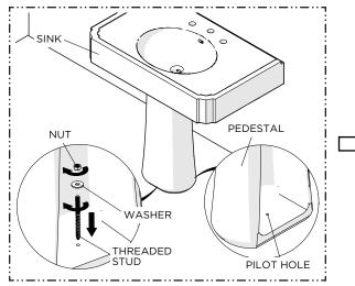
7. Dry fit the PEDESTAL to fit in front of the drain hole of the SINK. Mark where the hole is, drill, and secure the position using THREADED STUD, WASHER, and NUT.
