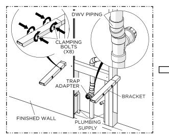
4. Once the level is set, tighten the CLAMPING BOLTS on both BRACKETS to secure the level. Ensure the PLUMBING SUPPLY and TRAP ADAPTER are properly installed before completing the FINISHED WALL installation.
