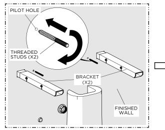
8. Install the M8 THREADED STUDS making sure the wood end is fully inserted into the FINISHED WALL, then apply adhesive silicone to the top surfaces of the SUPPORT BRACKETS.
