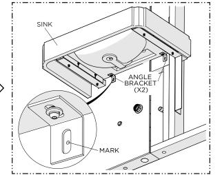
Dry fit the SINK with SUPPORT BRACKETS ensuring it is level. Mark the hole locations for the ANGLE BRACKETS then remove the SINK and drill pilot holes for M8 THREADED STUDS.
