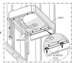
Dry-fit the SINK onto the BRACKETS and level it by adjusting the SET SCREWS at the bottom of each BRACKETS, Ensure the SINK'S weight is properly supported on the BRACKETS. Once aligned, remove the SINK and store it safely until the final installation.
