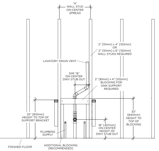
NOTE: This blocking scheme installs the sink top 34" [864mm] from the floor.
