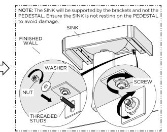
Place the SINK on BRACKETS against the FINISHED WALL. Install WASHERS and NUTS on THREADED STUDS and hand-tighten. Cut excess from STUDS, then securely tighten NUTS and SCREWS on ANGLE BRACKETS.
