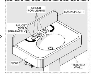
12. Turn on the water and operate the drain and FAUCET [sold separately] to ensure proper operation. Check all connections for leaks. If desired, a bead of caulk or clear silicone may be applied where the SINK contacts the FINISHED WALL.
