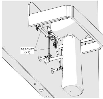
**NOTE:** The SINK will be supported by the brackets and not the PEDESTAL. Ensure the SINK is not resting on the PEDESTAL to avoid damage.
