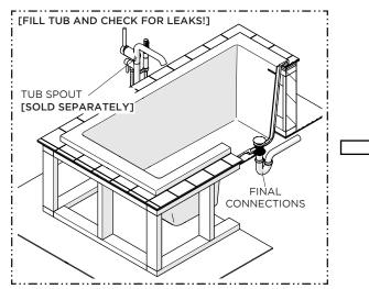
Make the final drain connections below the floor, then fill the BATHTUB up to the overflow hole and check for leaks. Ensure the drain and overflow are functioning.
