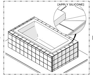
4. Complete the finished surface installation then apply silicone around the edges of the BATHTUB.
