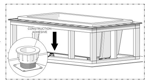
Remove the BATHTUB, apply construction adhesive to the bottom of each ADJUSTABLE FOOT, then place the TUB back into the framing structure and ensure it is level.
