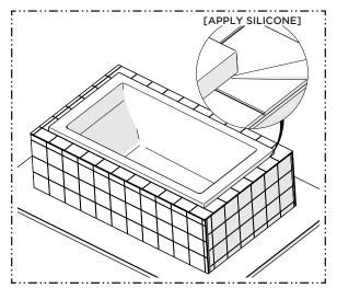
4. Complete the finished surface installation then apply silicone around the edges of the BATHTUB.
