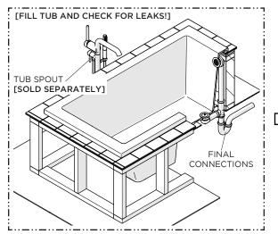
Make the final drain connections below the floor, then fill the BATHTUB up to the overflow hole and check for leaks. Ensure the drain and overflow are functioning.
