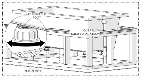
Dry-fit the BATHTUB into the framing structure to ensure the BATHTUB is level and ONLY supported by the ADJUSTABLE FOOT. Adjust the FOOT as needed.
