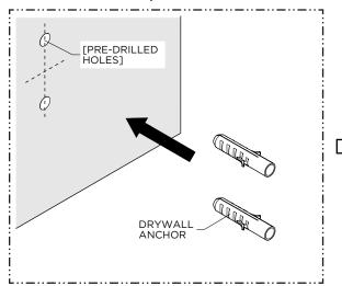
Using the previous marks as a reference, install the ANCHORS provided.
