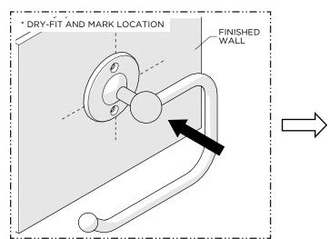
1. Dry-fit the product to the finished wall and mark the ideal location for installation.
