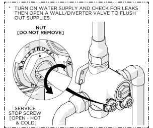
5. Turn on the water supplies then open the hot and cold SERVICE STOPS and open a diverter/wall valve to flush out the lines and check for leaks.
