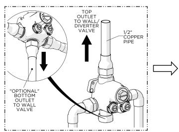
Run a 1/2" copper line from the top outlet and bottom outlet, if used, to a diverter/wall valve (sold separately) making sure to secure all piping and fittings.
