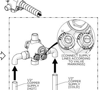
Run 1/2" copper supply lines to the proper height and depth of the VALVE INLETS making sure they are piped according to the VALVE markings and all piping and fittings are properly secured.
