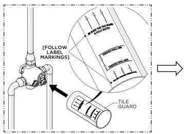
Following the label markings, firmly push the TILE GUARD onto the VALVE making sure it is FULLY seated.
