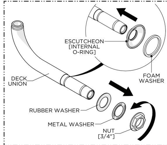
4. Remove the MOUNTING HARDWARE from each UNION then slide an ESCUTCHEON and FOAM WASHER onto each UNION making sure they are fully seated.
