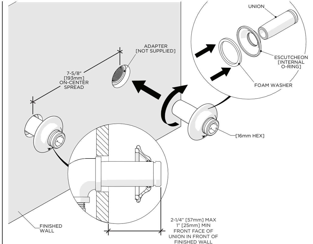
1. Verify the 7-5/8" [193mm] inlet supply spread then slide an ESCUTCHEON and FOAM WASHER onto each UNION.
