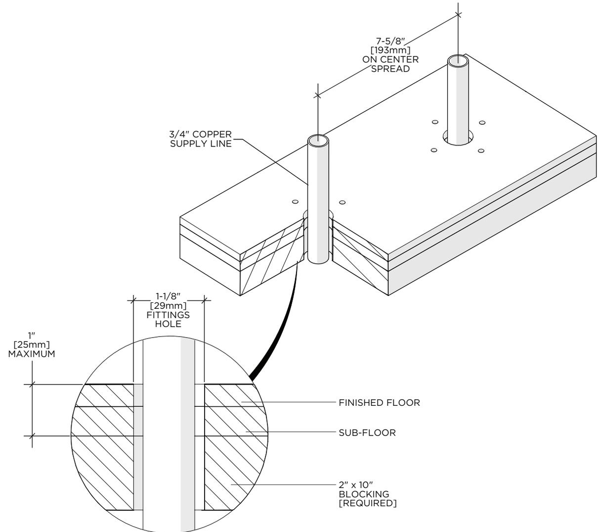
1. Rough-in and verify the 7-5/8" [193mm] inlet supply spread then refer to the INSTALLATION GUIDELINES provided **SEPARATELY** with the FLOOR UNIONS (Style No. UNUN32) to properly install the UNIONS.
