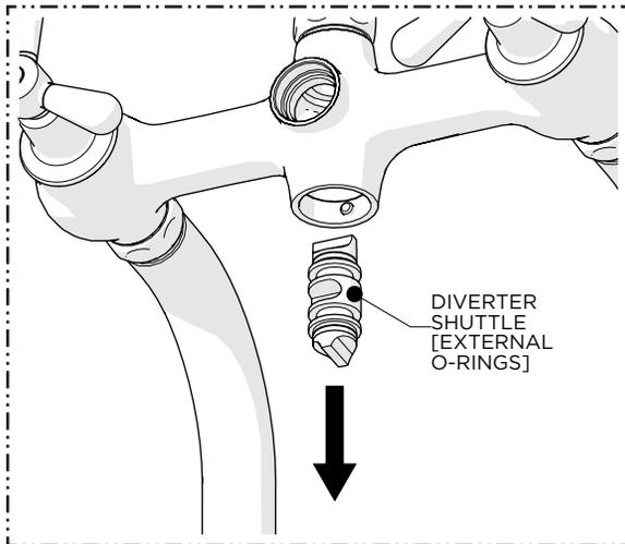
3. Remove the DIVERTER SHUTTLE from below.
