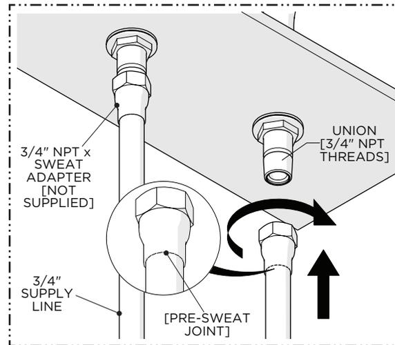
7. Pre-sweat 3/4" NPT x sweat ADAPTERS to the supply lines and let cool. Apply a thin coat of pipe thread sealant to the NPT threads on the UNIONS then thread and securely tighten the ADAPTERS onto the UNIONS.
