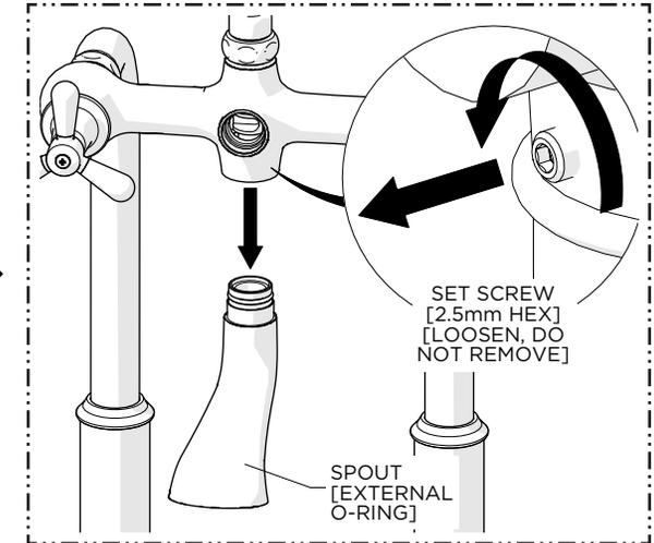
2. Loosen, but do **NOT** remove, the SET SCREW behind the TUB FILLER then remove the SPOUT.
