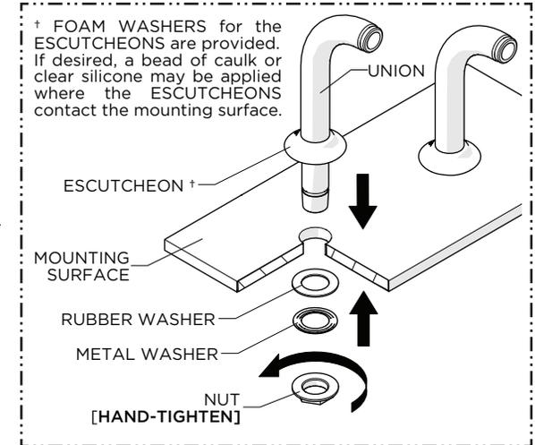
5. Insert each UNION through the hole on the mounting surface then re-install the MOUNTING HARDWARE and hand-tighten the NUT.
