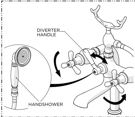
7. With water running, operate the DIVERTER HANDLE to ensure the HANDSHOWER functions properly.
