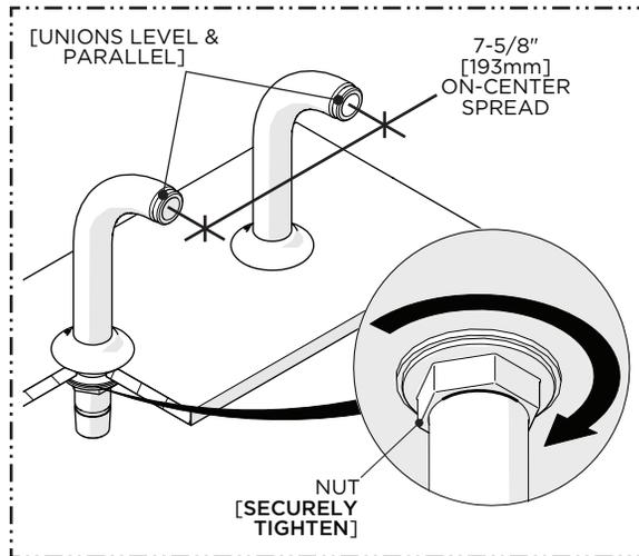
6. Verify the UNIONS are level, parallel to each other, and at the proper 7-5/8" [193mm] on-center spread then securely tighten the NUTS.
