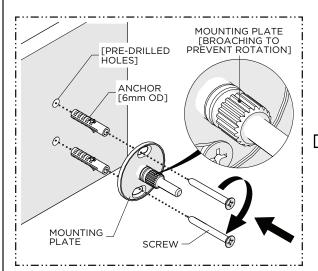
3. Using the previous marks as a reference, install the MOUNTING PLATE using the ANCHORS, if necessary, and SCREWS provided.
