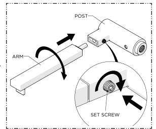
6. Rotate the ARM then re-insert it back into the POST. Ensure it is fully seated then securely tighten the SET SCREW.
