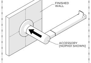
1. Dry-fit the ACCESSORY to the finished wall and mark the ideal location.
