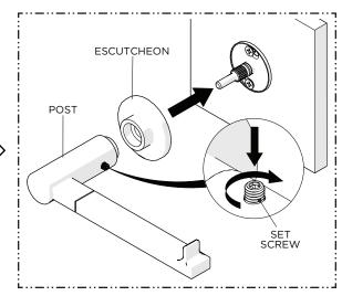
4. Slide the ESCUTCHEON and POST onto the MOUNTING PLATE then thread and securely tighten the SET SCREW.
