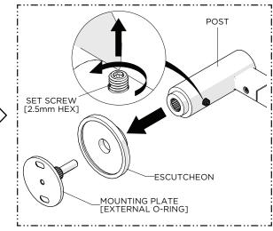
2. Loosen, but do NOT remove, the SET SCREW on the POST and remove the MOUNTING PLATE and ESCUTCHEON.
