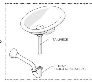
6. Make final P-TRAP (sold separately) connections and finish the installation then check for leaks.
