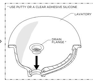
Set the DRAIN FLANGE into the LAVATORY (sold separately) using putty or a clear adhesive silicone.
