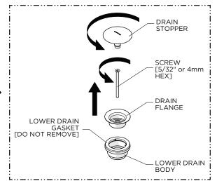
2. Remove the DRAIN STOPPER, SCREW, and DRAIN FLANGE from the LOWER DRAIN BODY.
