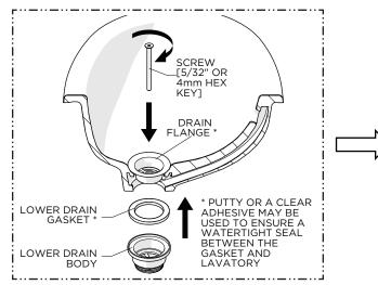
Using the LOWER DRAIN GASKET and SCREW provided, re-attach the LOWER DRAIN BODY to the FLANGE. Ensure the GASKET makes a full seal on the underside of the LAVATORY then securely tighten the SCREW.
