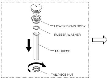
Remove the TAILPIECE NUT, TAILPIECE, and RUBBER WASHER from the LOWER DRAIN BODY.
