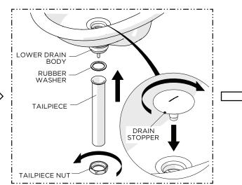
5. Re-install the DRAIN STOPPER and TAILPIECE using the WASHER and TAILPIECE NUT provided.
