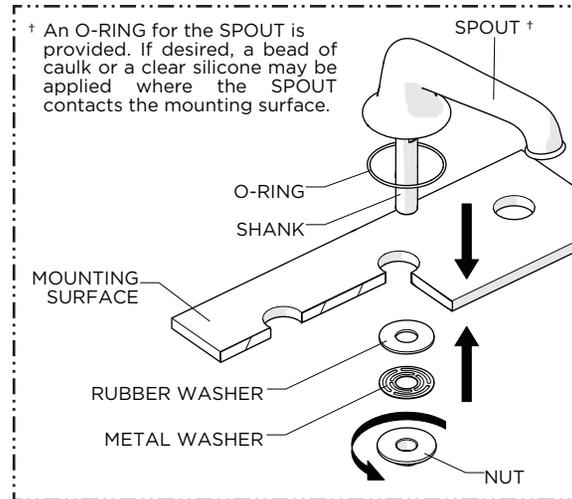
2. Insert the SHANK through the hole on the mounting surface making sure the O-RING provided is beneath the SPOUT then re-attach the RUBBER and METAL WASHERS and securely tighten the NUT.
