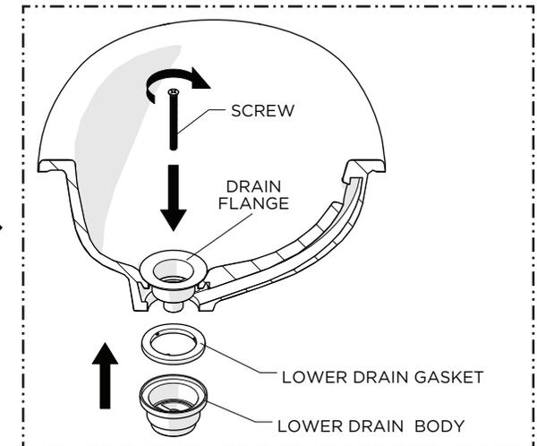
12. Insert the SCREW provided into the FLANGE then thread and securely tighten the SCREW into the LOWER DRAIN BODY making sure the LOWER DRAIN GASKET makes a full seal on the underside of the LAVATORY.
