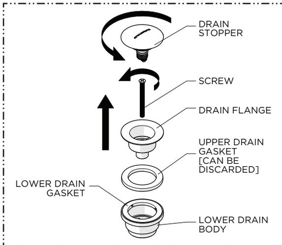
10. Remove the DRAIN STOPPER from the DRAIN FLANGE then unthread the SCREW from the LOWER DRAIN BODY.
