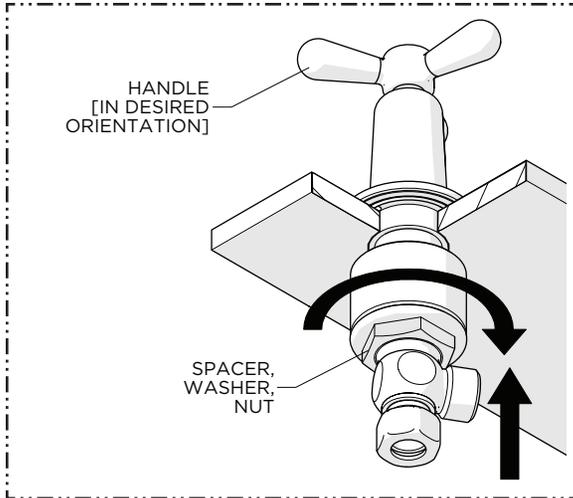
7. Ensure the HANDLE is in the desired orientation then thread and securely tighten the NUT against the underside of the mounting surface.
