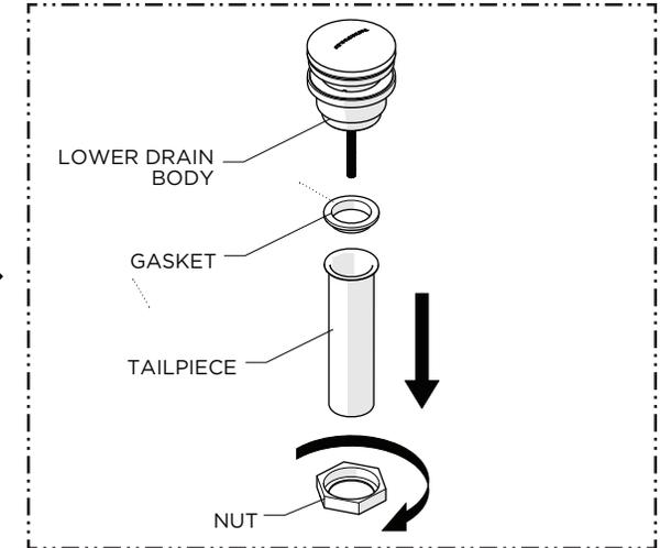
9. Unthread and remove the NUT, TAILPIECE, and GASKET from the LOWER DRAIN BODY.
