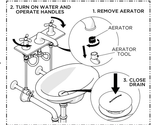
15. Remove the AERATOR, turn on the water to flush out the supply lines, inspect all connections for leaks and close the DRAIN to ensure it functions properly.
