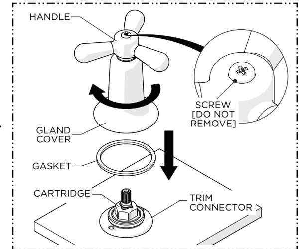
6. Using the GASKET provided, place the HANDLE over the CARTRIDGE STEM then thread and securely tighten the GLAND COVER onto the TRIM CONNECTOR.
