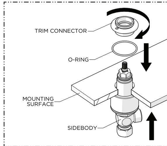
5. Using the O-RING provided, thread the TRIM CONNECTOR back onto the SIDEBODY until it stops then let it rest on the mounting surface.
