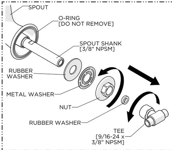
1. Remove the TEE, NUT, METAL WASHER, and RUBBER WASHER from the SPOUT SHANK.
