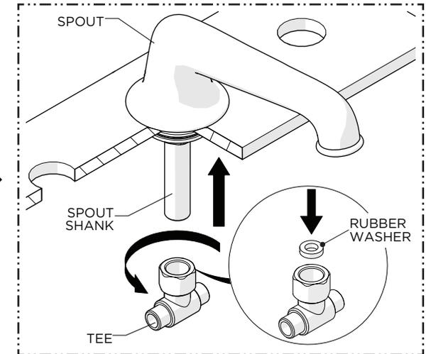
3. Thread and securely tighten the TEE onto the SHANK making sure to use the RUBBER WASHER provided.
