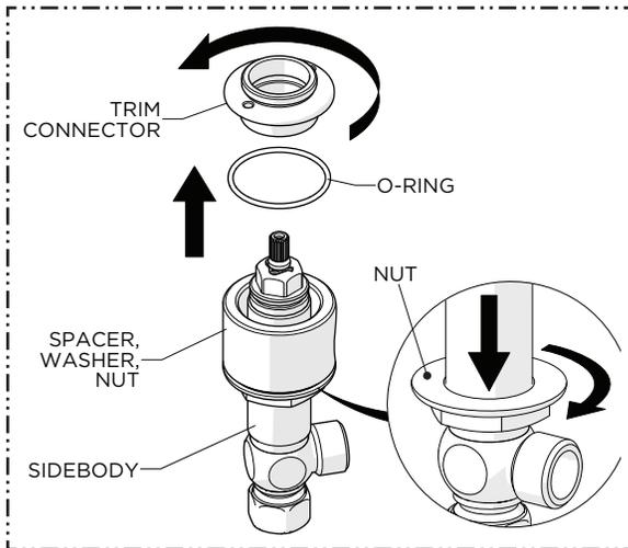
4. Unthread and remove the TRIM CONNECTOR with the O-RING beneath it then fully thread the NUT down the SIDEBODY.
