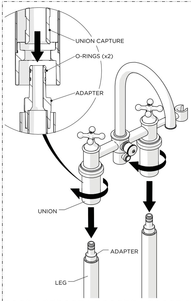
6. Align the UNIONS over the LEGS and slide the UNION CAPTURES onto the ADAPTERS then thread and securely tighten the UNIONS onto ADAPTERS.
