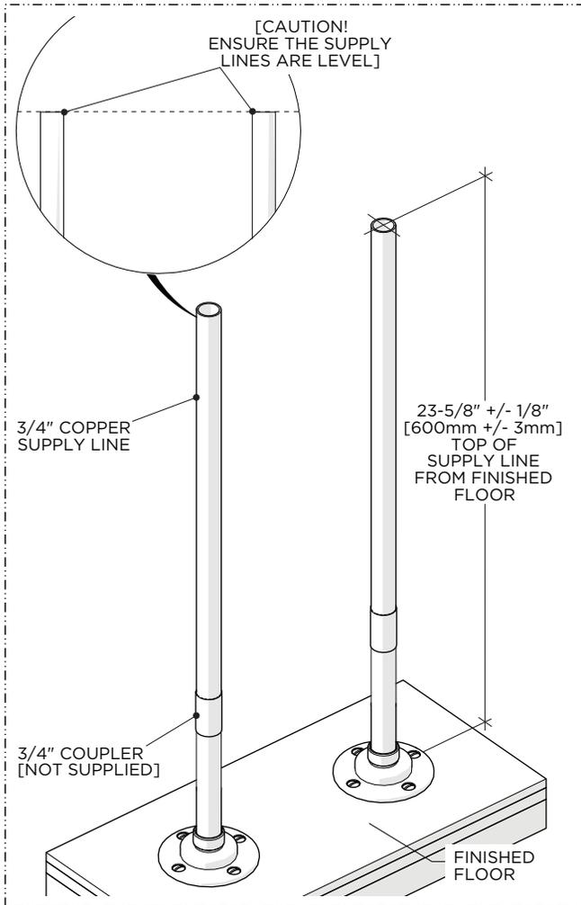
2. Using 3/4" COUPLERS (not supplied), extend the SUPPLY LINES to 23-5/8" [600mm] ± 1/8" [3mm] above the finished floor.
