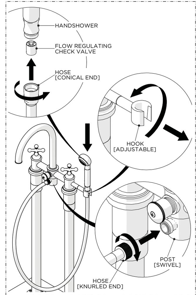
7. Thread and securely tighten the conical end of the HOSE to the HANDSHOWER and the knurled end to the POST at the base of the SPOUT then place the HANDSHOWER into the HOOK.
