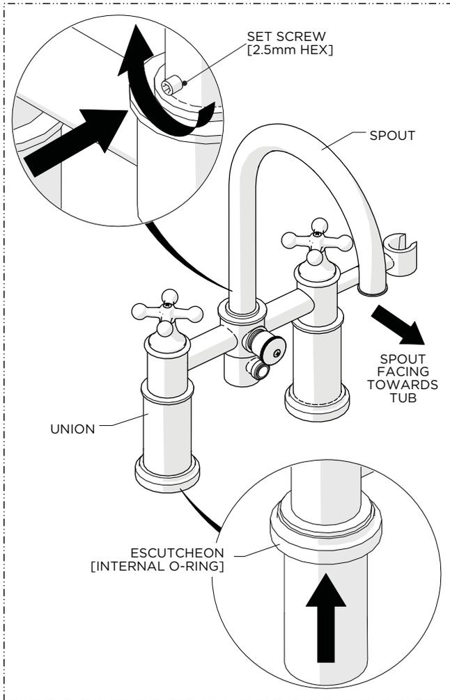
5. Align the SPOUT properly and securely tighten the SET SCREW at the base of the SPOUT then slide the ESCUTCHEONS up the UNIONS.
