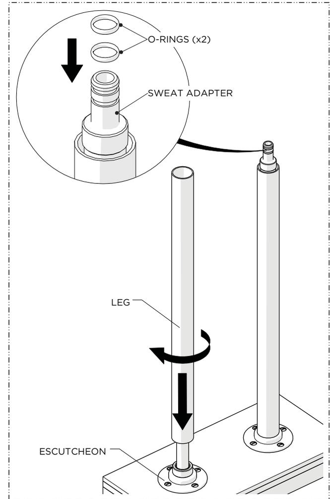
4. Thread and securely tighten the LEGS onto the ESCUTCHEONS then re-install the O-RINGS back onto the ADAPTER.
