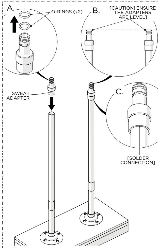
3. Remove the O-RINGS from the SWEAT ADAPTERS then place the ADAPTERS onto the SUPPLY LINES. Ensure the ADAPTERS are level then solder the inner diameter of each ADAPTER to the SUPPLY LINE.
