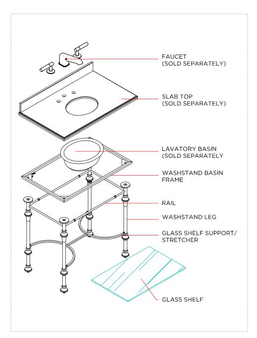
STYLE No. PEWS01 Pelham Four Leg Single Washstand Packaged with Sink and Slab Top  $39" \times 24" \times 38"$
