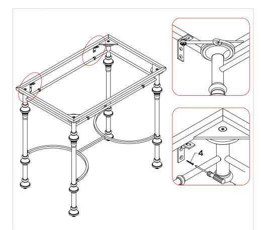
Slightly loosen the metal brackets attached to the back of the Washstand basin frame. At your desired location, secure the washstand with screws (4) provided.
