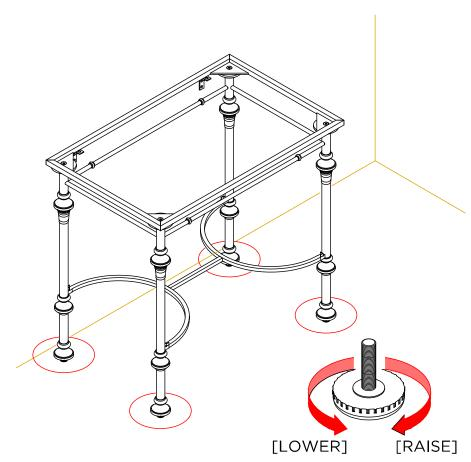
• From your prepared location, pre-set the unit against the wall, examine the alignment of the washstand if leveling is necessary. If needed, slightly tilt the washstand and turn the head of the levelers clockwise to raise the furniture and counter-clockwise to lower it. Adjust all levelers until the correct level or flatness is achieved.
