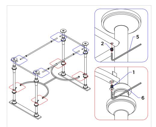
Arrange the washstand Legs, Frame, Rails, and Stretcher in place with the hardware cavities facing inside. Set both legs in an upright position and leave enough space for the Rails and Stretcher assembly.
