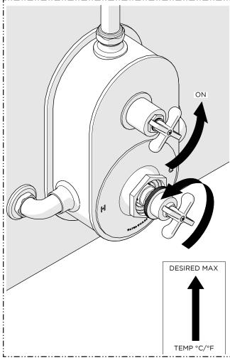
17. With water running, rotate the CARTRIDGE STEM on the THERMOSTATIC VALVE to adjust the temperature to the maximum desired bathing temperature, verified with a thermometer. Turn the water off and make sure not to change this setting.
