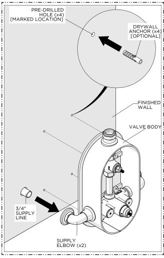
Remove the VALVE BODY and, using the previous marks, pre-drill holes (pilot holes) to accommodate the MOUNTING SCREWS. If necessary, install the DRYWALL ANCHORS provided where blocking is not installed.
