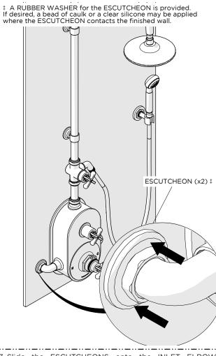
23. Slide the ESCUTCHEONS onto the INLET ELBOWS against the finished wall.
