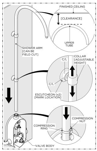
Fully insert the SHOWER ARM into the top of the VALVE BODY making sure the ESCUTCHEON for the SUPPORT POST sits flush against the finished wall and there is enough clearance between the top of the SHOWER ARM and the finished ceiling.
