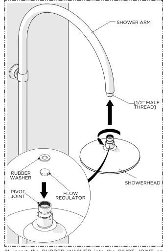
21. Insert the RUBBER WASHER into the PIVOT JOINT on the SHOWERHEAD (packaged separately) then thread and securely tighten the PIVOT JOINT onto the SHOWER ARM
