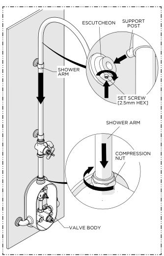
11. Fully insert the SHOWER ARM into the top of the VALVE BODY making sure the SUPPORT POST is fully inserted into the ESCUTCHEON, thread and securely tighten the SET SCREW. Thread and securely tighten the COMPRESSION NUT on the SHOWER ARM to the VALVE.
