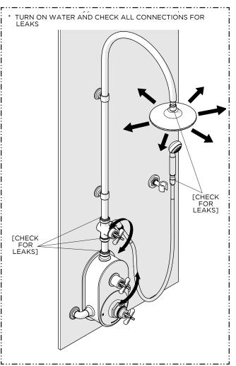
22. Turn on the water and operate the SHOWERHEAD to ensure it pivots and functions properly.
