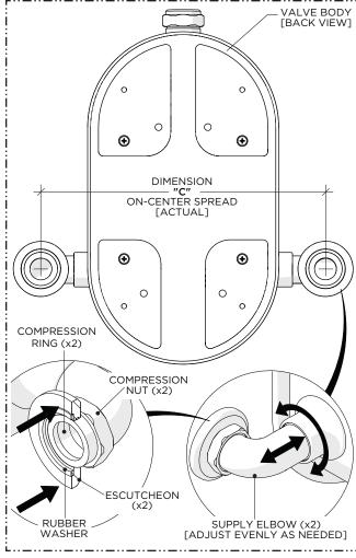
Push the ESCUTCHEONS against the COMPRESSION NUTS then measure the on-center spread of the SUPPLY ELBOWS (DIMENSION C).
