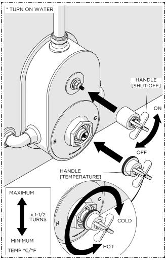
Turn on the water supply and open the SHUTOFF VALVE to run water through the THERMOSTATIC VALVE and check for leaks.
