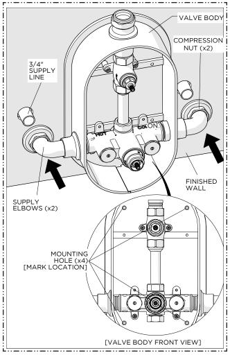
Dry-fit the SUPPLY ELBOWS onto the SUPPLY LINES making sure the VALVE BODY sits flush against the finished wall then mark the location of the MOUNTING HOLES (x4).
