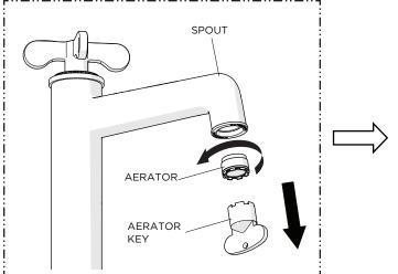
Remove the AERATOR from the SPOUT using the tool provided.
