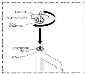
4. With the HANDLE held horizontally thread the RING ADAPTER into the SPOUT until snug.
