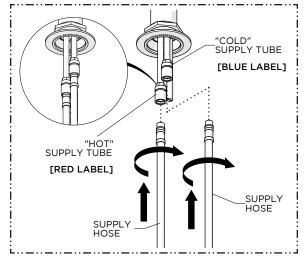
2. Thread and securely tighten the SUPPLY HOSES onto the SUPPLY TUBES on the SPOUT.
