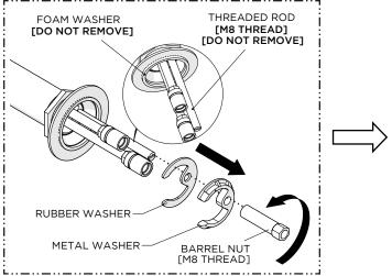
Remove the BARREL NUT, METAL WASHER, and RUBBER WASHER from the THREADED ROD.
