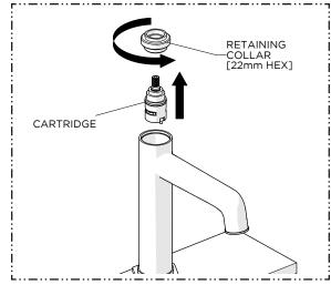
Unthread and remove the RETAINING COLLAR then pull the CARTRIDGE out.
