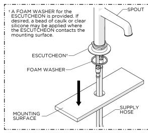
Insert the SUPPLY HOSES through the hole on the mounting surface making sure the FOAM WASHER provided is beneath the ESCUTCHEON.
