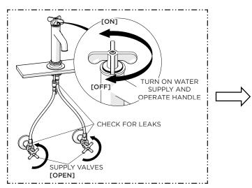
10. Turn on the water supply to flush out the supply lines and inspect all connections for leaks.
