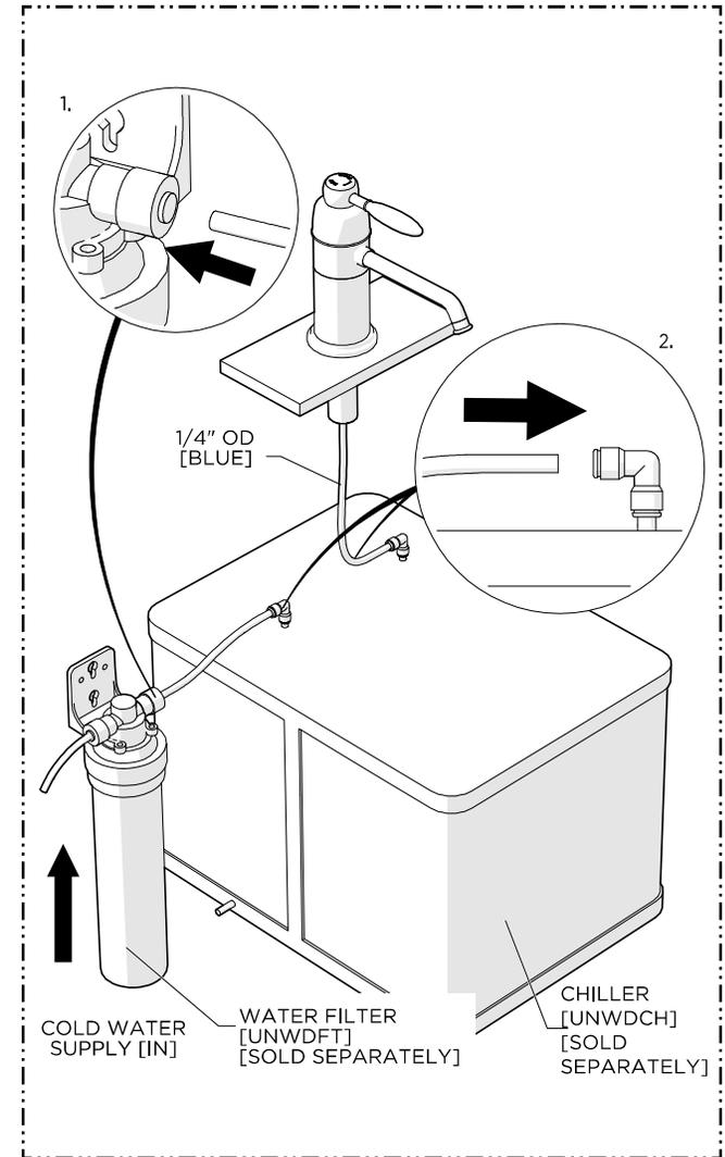
3. Insert the BLUE 1/4" O.D. TUBE from the SPOUT into the CHILLER [SOLD SEPARATELY] 1/4" OUTLET. Insert 1/4" O.D. TUBE [SUPPLIED WITH THE FILTER] from the WATER FILTER OUTLET [SOLD SEPARATELY] into the CHILLER INLET.
