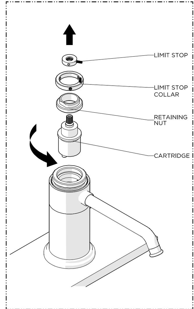
2. Remove the LIMIT STOP and the LIMIT STOP COLLAR then unthread the RETAINING NUT and remove the CARTRIDGE.
