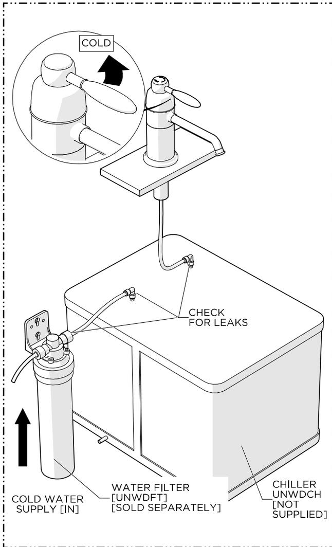
4. Turn on the water to flush out any debris in the supply lines, operate the HANDLE and SPOUT to ensure they function properly and inspect all connection for leaks.
