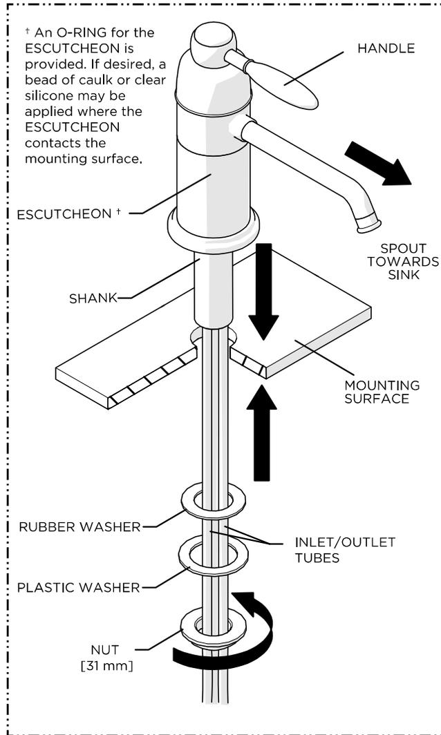
2. Insert the INLET/OUTLET TUBES and SHANK through the hole on the mounting surface. Place HANDLE in off position, line up SPOUT with HANDLE and position SPOUT over sink in desired location then re-attach the WASHERS and securely tighten the NUT.
