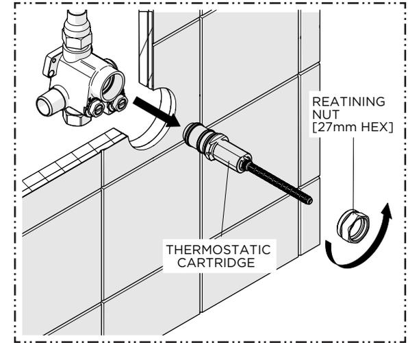
8. Unthreaded the **RETAINING NUT** and remove the **CARTRIDGE**.
