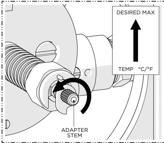
12. With water running, rotate the ADAPTER STEM to adjust the temperature to the **maximum** desired bathing temperature, verified with a thermometer, then turn the water off and make sure **NOT** to change this setting.
