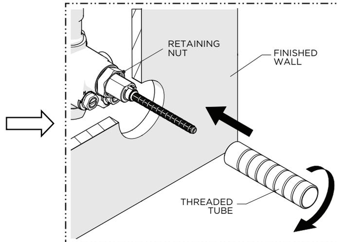
4. Thread the THREADED TUBE into the RETAINING NUT until it stops.
