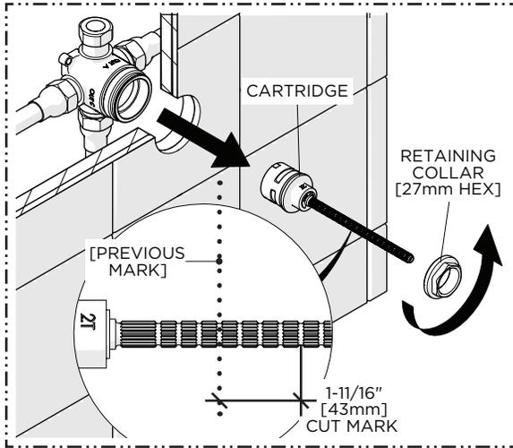
4. Unthread the RETAINING COLLAR and remove the CARTRIDGE then cut the CARTRIDGE STEM 1-11/16" [43mm] **in front** of the previous mark so the STEM will protrude 1-11/16" [43mm] from the finished wall surface.
