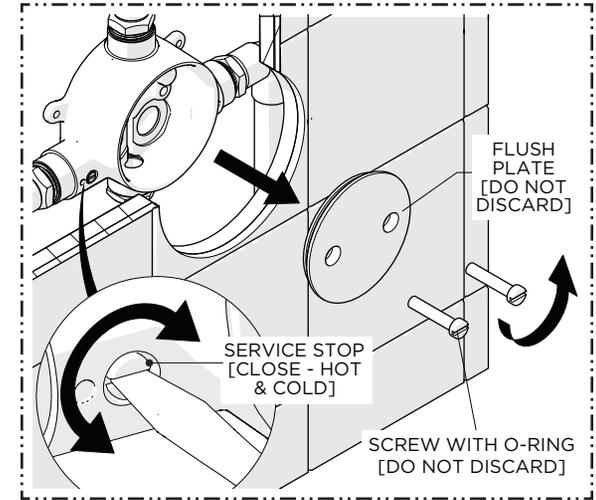
1. Turn on the water supplies then remove the TILE GAURDS from the VALVE and **OPEN** the SERVICE STOPS (hot & cold) to flush out the lines.
