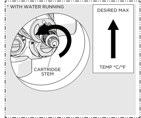
14. With water running rotate the CARTRIDGE STEM to adjust the temperature to the **maximum** desired bathing temperature, verified with a thermometer, then turn the water off and make sure **NOT** to change this settings.
