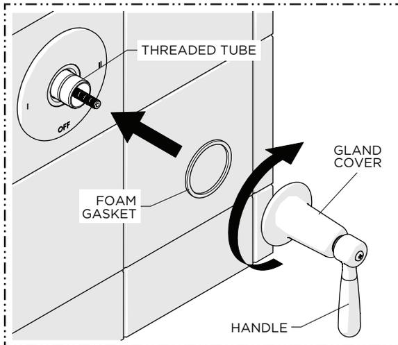
7. Firmly holding the DIVERTER PLATE against the finished wall and using the FOAM GASKET provided, thread and securely tighten the GLAND COVER onto the THREADED TUBE.
