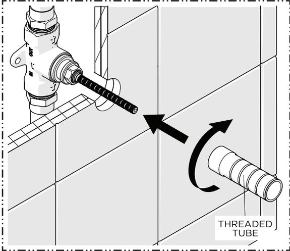
11. Thread and securely tighten the THREADED TUBE back onto the CARTRIDGE until it stops.
