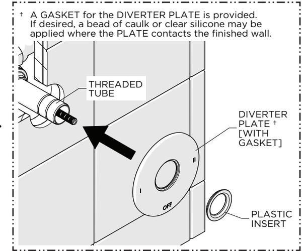
6. Using the PLASTIC INSERT provided, slide the DIVERTER PLATE over the THREADED TUBE.
