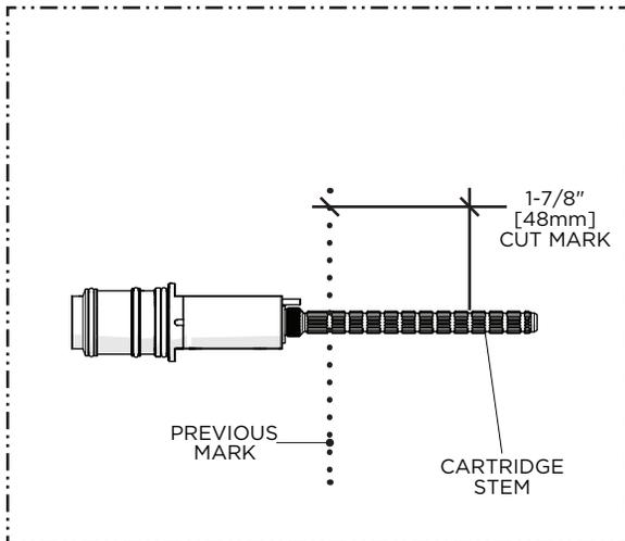
9. Carefully cut the **CARTRIDGE STEM** 1-7/8" [48mm] **in front** of the previous mark so the **STEM** will protrude 1-7/8" [48mm] from the finished wall surface.
