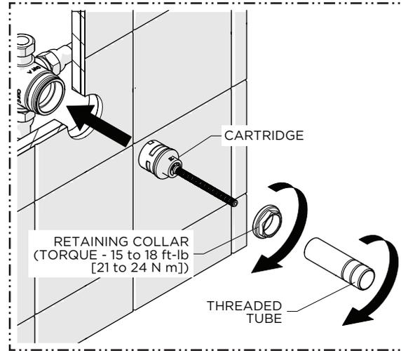
5. Re-insert the CARTRIDGE then thread and securely tighten the RETAINING COLLAR to the specified torque setting shown.
