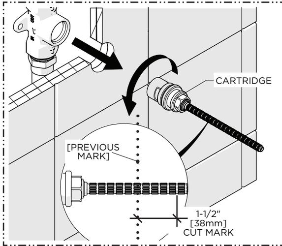
4. Remove the CARTRIDGE using a 21/32" [17mm] shower valve socket wrench (not supplied) then cut the CARTRIDGE STEM 1-1/2" [38mm] in front of the previous mark so the STEM will protrude 1-1/2" [38mm] from the finished wall surface.
