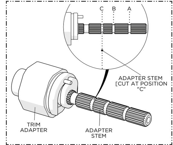
8. Before installing the TRIM ADAPTER cut the ADAPTER STEM at position "C" as shown.
