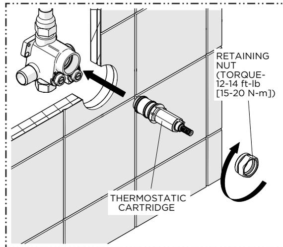
10. Insert the **CARTRIDGE** back into the **VALVE BODY** then thread and securely tighten the **RETAINING NUT** to the specified torque settings shown.
