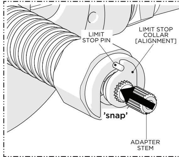
13. Slide the LIMIT STOP COLLAR back down the ADAPTER STEM making sure to properly align it with the LIMIT STOP PIN and pressing down firmly.
