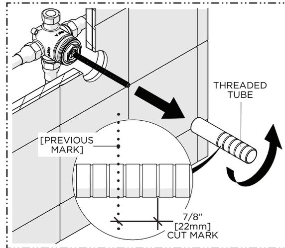
2. Remove the THREADED TUBE then cut it 7/8" [22mm] in front of the previous mark so the TUBE will protrude 7/8" [22mm] from the finished wall surface.
