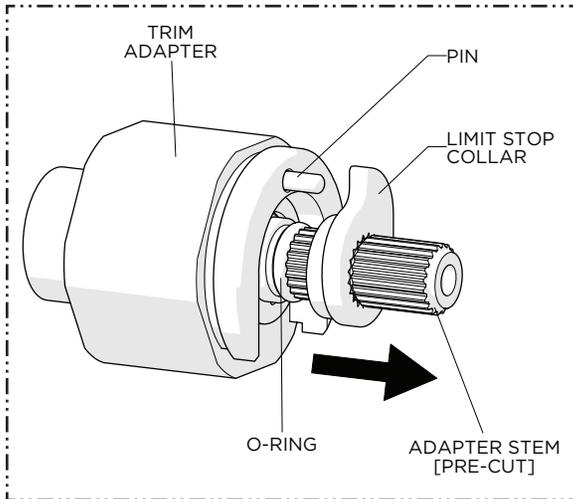
9. After cutting the ADAPTER STEM, pull the LIMIT STOP COLLAR up the STEM so it no longer contacts the PIN. The COLLAR must be unseated to allow the TRIM ADAPTER to thread properly onto the THREADED TUBE.
