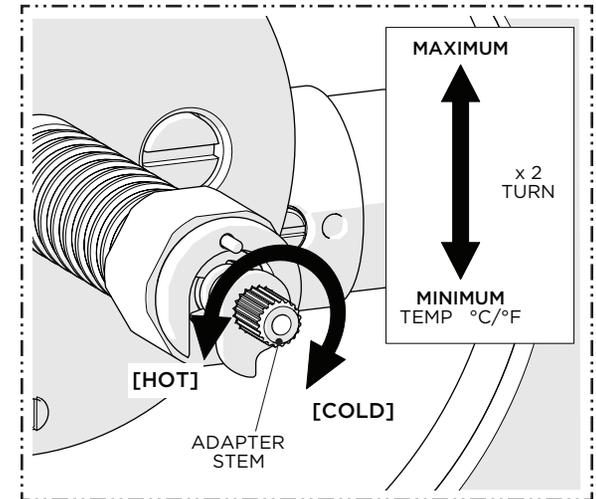
11. Open a DIVERTER or VOLUME CONTROL VALVE then slowly rotate the ADAPTER STEM clockwise to attain full hot then rotate it counter-clockwise to attain full cold. Verify that a full range of temperatures exists.
