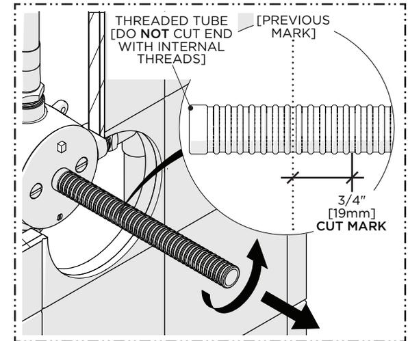
5. Remove the THREADED TUBE then cut it 3/4" [19mm] in front of the previous mark.
