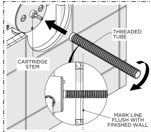
4. Fully thread the THREADED TUBE onto the CARTRIDGE STEM and mark the TUBE where it protrudes past the finished wall.
