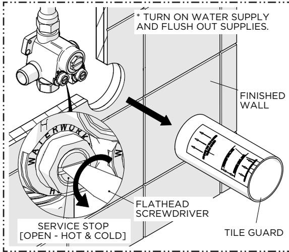
1. Turn on the water supplies then remove the TILE GAURD from the VALVE and **OPEN** the SERVICE STOPS (hot & cold) to flush out the lines.
