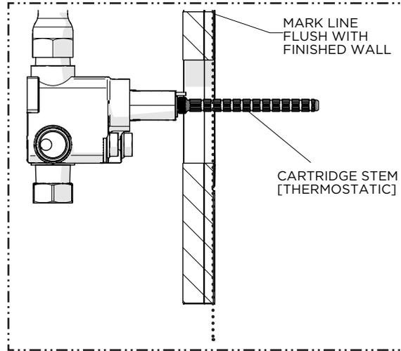
7. Mark the **CARTRIDGE STEM** where it protrudes past the finished wall.
