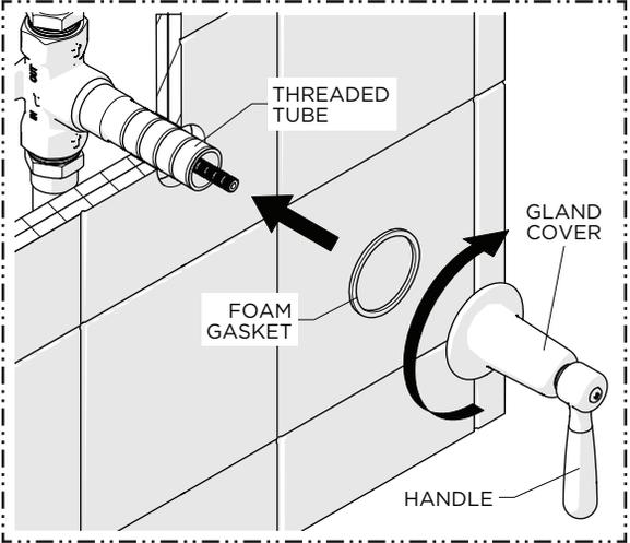
12. Using the FOAM WASHER provided and the HANDLE in the desired orientation, thread and securely tighten the GLAND COVER onto the THREADED TUBE.
