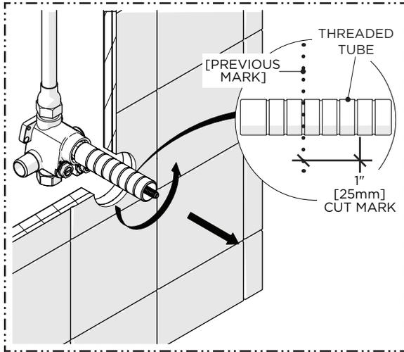
6. Remove the **THREADED TUBE** then cut it 1" [25mm] **in front** of the previous mark so the **TUBE** will protrude 1" [25mm] from the finished wall surface.
