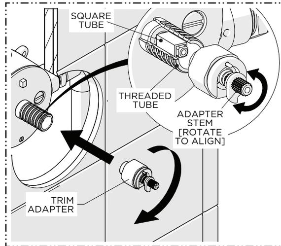
10. Thread the TRIM ADAPTER onto the THREADED TUBE until it stops.
