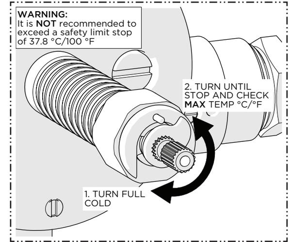
14. Turn the ADAPTER STEM clockwise to full cold then counter-clockwise until it stops and verify the **maximum** desired bathing temperature set in the previous step.
