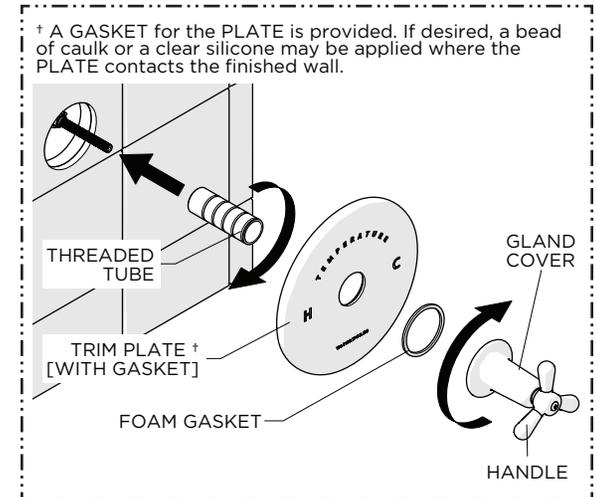
17. Thread the THREADED TUBE back into the RETAINING NUT until it stops, slide the TRIM PLATE over the TUBE and firmly hold it against the finished wall then thread and securely tighten the HANDLE onto the TUBE making sure to use the GASKET provided.
