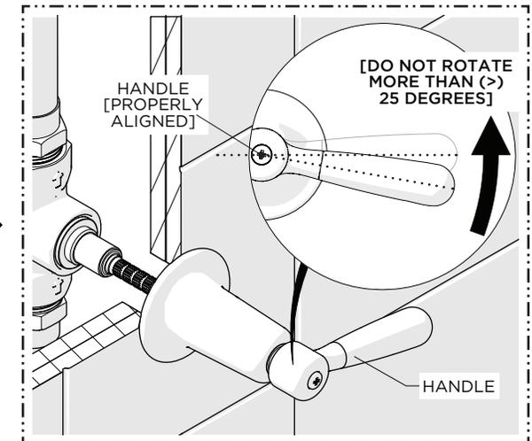
9. **If needed**, carefully continue to rotate the HANDLE counter-clockwise to obtain the proper alignment. Do **NOT** rotate/unthread the CARTRIDGE more than 25 degrees.
