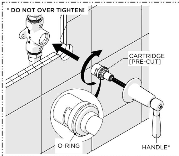
7. Using the HANDLE, thread the CARTRIDGE back into the VALVE until there is **NOTICEABLE** resistance.
