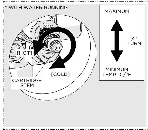
13. Open a DIVERTER or VOLUME CONTROL VALVE then slowly rotate the CARTRIDGE STEM clockwise to attain full hot then counter-clockwise to attain full cold. Verify that a full range of temperatures exists.
