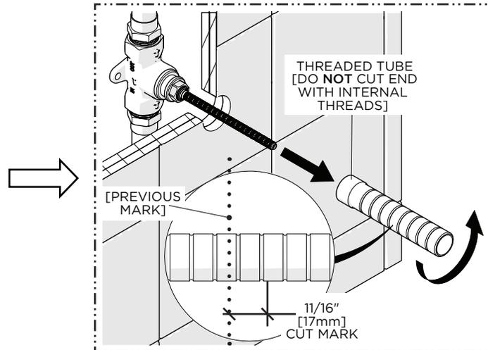
2. Remove the THREADED TUBE then cut it 1/16" [17mm] in front of the previous mark so the TUBE will protrude 1/16" [17mm] from the finished wall surface.
