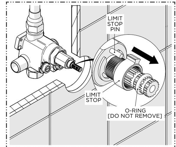
11. Slide the **O-RING** and **LIMIT STOP** on the **THERMOSTATIC CARTRIDGE** up the **STEM**.
