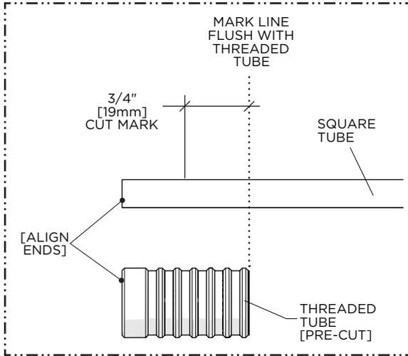
6. Align the pre-cut THREADED TUBE with the SQUARE TUBE then mark and cut the SQUARE TUBE 3/4" [19mm] shorter than the THREADED TUBE.
