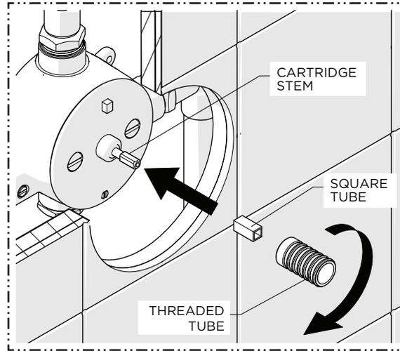
7. Slide the SQUARE TUBE onto the CARTRIDGE STEM then thread the THREADED TUBE onto the STEM until it stops.
