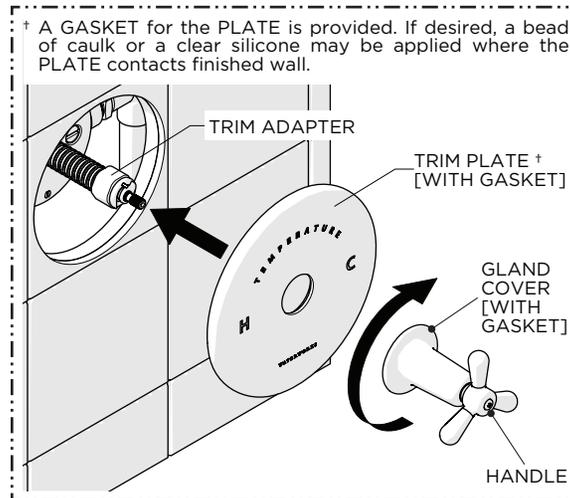
15. Slide the TRIM PLATE over the TRIM ADAPTER and firmly hold it against the finished wall then securely tighten the HANDLE onto the ADAPTER making sure to use the GASKET provided.
