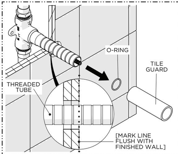
1. Remove the TILE GUARD when ready to install the TRIM then mark the THREADED TUBE where it protrudes past the finished wall.
