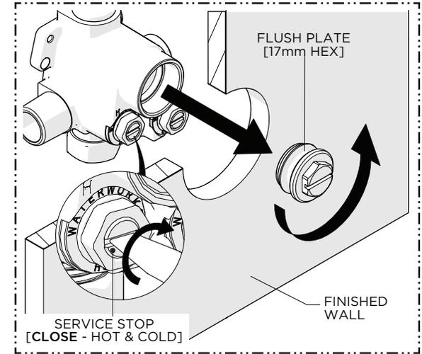
2. After the lines have been fully flushed, **CLOSE** the SERVICE STOPS (hot & cold) then unthreaded and remove the FLUSH PLATE.
