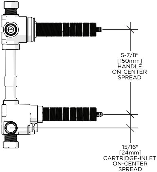
➤ The **THERMOSTATIC VALVE** only mixes hot and cold water. It does not have volume or shut-off capabilities. Mixed water flows out at a fixed volume to the **INTEGRATED TWO WAY DIVERTER WITH SHUTOFF VALVE** which has 3 positions.
