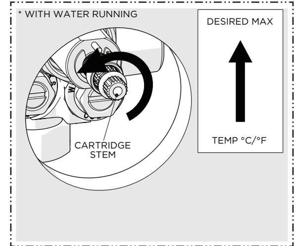
14. With water running, rotate the STEM to adjust the temperature to the **maximum** desired bathing temperature, verified with a thermometer, then close the DIVERTER VALVE and make sure **NOT** to change this setting.
