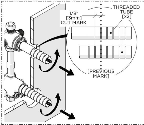
6. Remove the TUBES and cut them 1/8" [3mm] behind the previous mark so the TUBES will be 1/8" [3mm] below or recessed into the finished wall surface.
