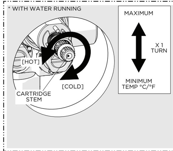
13. With water running, slowly rotate the THERMOSTATIC CARTRIDGE STEM clockwise to attain full cold then rotate it counterclockwise to attain full hot. Verify that a full range of temperatures exists.
