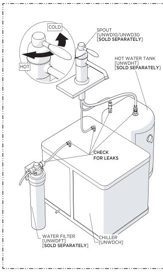
6. Turn on the water to flush out any debris in the supply lines, operate the HANDLE and SPOUT to ensure they function properly and inspect all connection for leaks.
