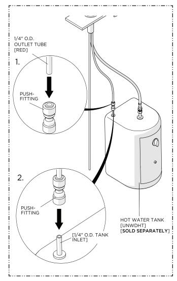
Insert the RED 1/4" O.D. OUTLET TUBE from the SPOUT into the PUSH-FITTING then connect the FITTING to the 1/4" O.D. TANK INLET.
