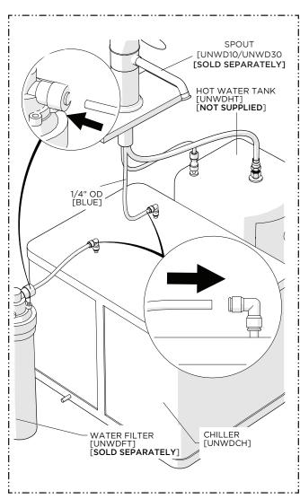
5. Insert the BLUE 1/4" O.D. TUBE from the SPOUT into the CHILLER 1/4" OUTLET. Insert 1/4" O.D. TUBE [SUPPLIED WITH THE FILTER] from the WATER FILTER OUTLET [SOLD SEPARATELY] into the CHILLER INLET.
