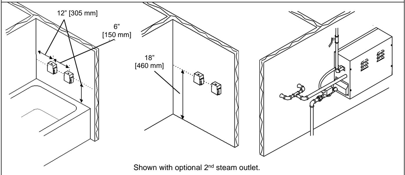
**5. INSTALL PRESSURE RELIEF SAFETY VALVE:** Install the pressure relief valve into its port on the generator. Install the safety valve within 6" [150] mm of the generator. Run a 3/4" copper line from the valve to a gravity flow drain. The pressure relief valve outlet must drain in accordance with local and national codes.
