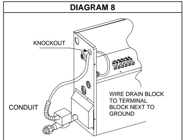
**2. ELECTRICAL INFORMATION** The steamers are available in 2 basic versions, one for 208V (intended for 208VAC single and three phase for North American use) and 240V (intended for all other installations. The 240V models are rated at 240VAC and may be used on 208 to 240V single phase Line-to-Line or 208 to 240V~N (Line-to-Neutral) or 208V to 240V three phase Delta without Neutral or for Y-connected three phase 380 to 415V~N3.
