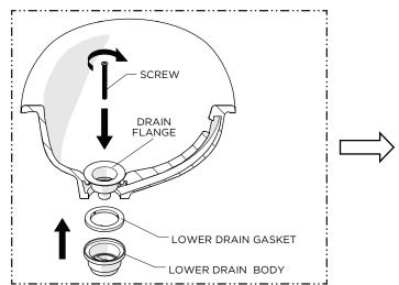
7. Insert the SCREW provided into the FLANGE then thread and securely tighten the SCREW into the LOWER DRAIN BODY making sure the LOWER DRAIN GASKET makes a full seal on the underside of the LAVATORY.
