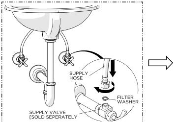
10. Connect the SUPPLY HOSES to the SUPPLY VALVES (sold separately), making sure to use the FILTER WASHERS provided.
