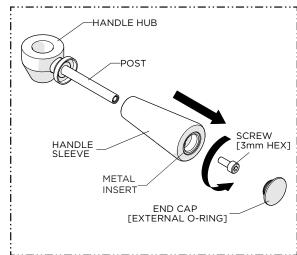
Remove the END CAP, then unthread and remove the SCREW from the POST, then remove the HANDLE SLEEVE from the POST.
