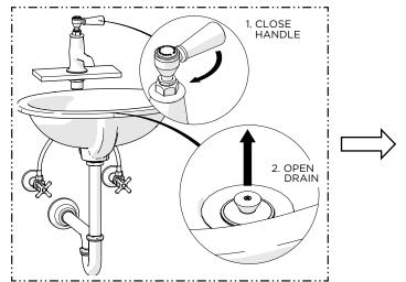
13. Close the HANDLE then open the DRAIN to drain the water.
