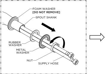
Remove the NUT, METAL WASHER, and RUBBER WASHER from the SPOUT SHANK.
