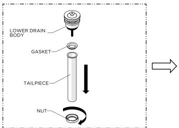
4. Unthread and remove the NUT, TAILPIECE, and GASKET from the LOWER DRAIN BODY.
