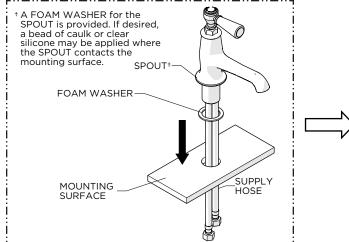
Insert the SUPPLY HOSES through the hole on the mounting surface making sure the FOAM WASHER provided is beneath the SPOUT.
