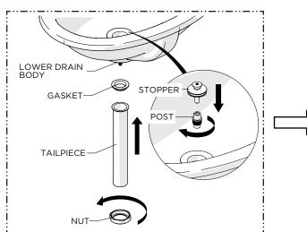
8. Re-install the POST, DRAIN STOPPER, and TAILPIECE using the GASKET and NUT provided.
