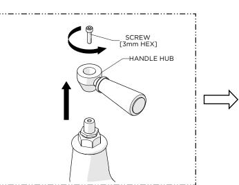
2. Unthread and remove the SCREW from the HANDLE HUB and then remove the HANDLE.
