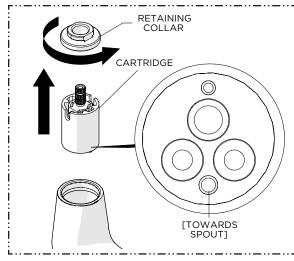
Unthread and remove the RETAINING COLLAR then pull the CARTRIDGE out.
