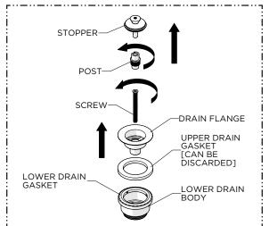
Remove the DRAIN STOPPER and POST from the DRAIN FLANGE then unthread the SCREW from the LOWER DRAIN BODY.
