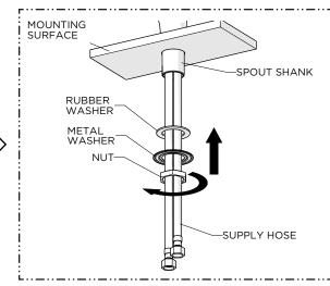
Slide the RUBBER and METAL WASHERS back onto the SPOUT SHANK then thread and securely tighten the NUT onto the SHANK.
