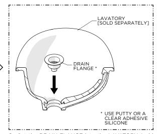
Set the DRAIN FLANGE into the LAVATORY (sold separately) using putty or a clear silicone.
