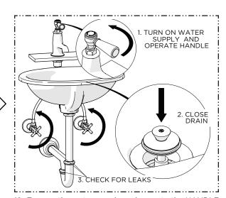
12. Turn on the water supply and operate the HANDLE to flush out the supply lines. Inspect all connections for leaks then close the DRAIN to ensure it functions properly.
