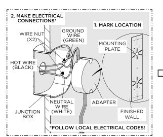
Dry fit and mark the screw locations on the finished wall. Use WIRE NUTS to connect the HOT (BLACK) and NEUTRAL (WHITE) wires.
