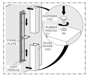
4. Take the GLASS SHADE and carefully slide it onto the LIGHT MODULE, ensuring it rests on the FIXING PLATE. Place the RUBBER PAD, centering it over the top/bottom hole on the GLASS SHADE, and secure it with the FASTENER provided and repeat the same steps for the other side.
