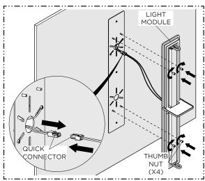
3. Connect the QUICK CONNECTOR from the ADAPTER to the QUICK CONNECTOR on the LIGHT MODULE. Position the LIGHT MODULE onto the MOUNTING PLATE ensuring the screw holes align. Fasten the THUMB NUTS to the LIGHT MODULE screws ensuring they are fully tightened.
