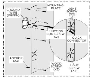
Insert the ADAPTER into the JUNCTION BOX, secure the BRACKET with the provided ANCHORS and SCREWS, ensuring the ADAPTER QUICK CONNECTOR passes through the BRACKET center hole. Attach the MOUNTING PLATE and connect the GROUND wire to the JUNCTION BOX SCREWS.
