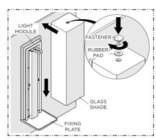
4. Take the GLASS SHADE and carefully slide it onto the LIGHT MODULE, ensuring it rests on the FIXING PLATE. Place the RUBBER PAD, centering it over the top hole on the GLASS SHADE, and secure it with the FASTENER provided.
