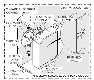
Dry fit and mark the screw locations on the finished wall. Use WIRE NUTS to connect the HOT (BLACK) and NEUTRAL (WHITE) wires.
