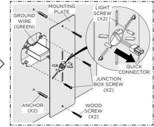
Insert the ADAPTER into the JUNCTION BOX, secure the BRACKET with the provided ANCHORS and SCREWS, ensuring the ADAPTER QUICK CONNECTOR passes through the BRACKET center hole. Attach the MOUNTING PLATE and connect the GROUND wire to the JUNCTION BOX SCREWS.
