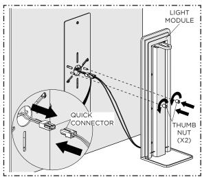
3. Connect the QUICK CONNECTOR from the ADAPTER to the QUICK CONNECTOR on the LIGHT MODULE. Position the LIGHT MODULE onto the MOUNTING PLATE ensuring the screw holes align. Fasten the THUMB NUTS to the LIGHT MODULE screws ensuring they are fully tightened.
