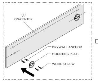
Using the previous marks as a reference, install the MOUNTING PLATES using the SCREWS and ANCHORS provided.
