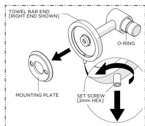
Loosen, but do NOT remove, the SET SCREW on the bottom of each TOWEL BAR END using a 2mm HEX KEY and remove the MOUNTING PLATES.
