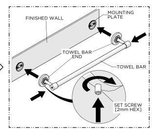
Holding the ENDS and BAR together, place both ENDS over the MOUNTING PLATES and securely tighten the SET SCREWS.
