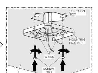
Route the ELECTRICAL WIRES through the center hole of the MOUNTING BRACKET and secure the MOUNTING BRACKET to the JUNCTION BOX with the provided SCREWS.
