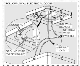
Use WIRE NUTS to connect the HOT (BLACK) and NEUTRAL (WHITE) WIRES from the JUNCTION BOX to the HOT (BLACK) and NEUTRAL (WHITE) WIRES of the FIXTURE, and connect the GROUND WIRE (GREEN) from the JUNCTION BOX to the GROUND NUT on the MOUNTING BRACKET.
