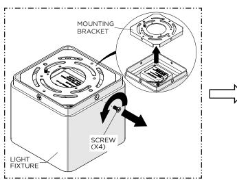
1. Unthread the SCREWS and carefully remove the MOUNTING BRACKET from the LIGHT FIXTURE.
