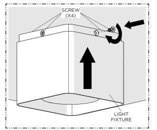
Once the wiring is complete, attach the LIGHT FIXTURE to the MOUNTING BRACKET using the provided SCREWS. Verify the FIXTURE is securely mounted.
