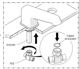
Thread and securely tighten the TEE onto the SHANK making sure to use the FIBER WASHER provided.
