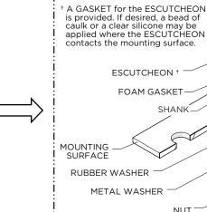
2. Insert the SHANK through the hole on the mounting surface, making sure the FOAM GASKET is beneath the ESCUTCHEON, then re-install the LOWER DECK WASHERS and securely tighten the NUT.
