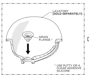
14. Set the DRAIN FLANGE into the LAVATORY (sold separately) using putty or a clear silicone.
