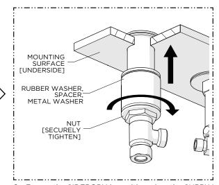
6. Ensure the SIDEBODY is positioned so the SUPPLY HOSE can be easily connected to the TEE then thread and securely tighten the NUT against the underside of the mounting surface.
