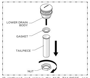
12. Unthread and remove the NUT, TAILPIECE, and GASKET from the LOWER DRAIN BODY.
