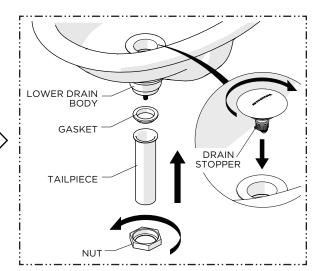
Re-install the DRAIN STOPPER and TAILPIECE using the GASKET and NUT provided.
