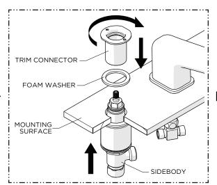
5. Using the FOAM WASHER provided, thread the TRIM CONNECTOR back onto the SIDEBODY until snug then let it rest on the mounting surface.
