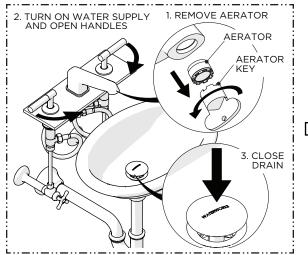
18. Remove the AERATOR, turn on the water supply and open the HANDLES to flush out the supply lines, and inspect all connections for leaks then close the DRAIN to ensure it functions properly.
