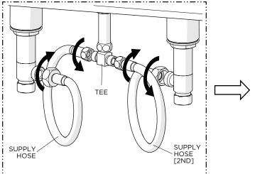
11. Connect the SIDEBODIES to the TEE using the SUPPLY HOSES provided. Securely tighten the HOSES and ensure they are not pinched/kinked.
