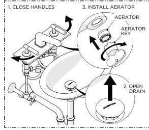
19. Close the HANDLES, open the DRAIN to drain the water, and re-install the AERATOR.
