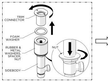
4. Unthread and remove the TRIM CONNECTOR and FOAM WASHER from the SIDEBODY then fully thread the NUT down the SIDEBODY.
