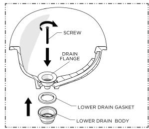
15. Insert the SCREW provided into the FLANGE then thread and securely tighten the SCREW into the LOWER DRAIN BODY making sure the LOWER DRAIN GASKET makes a full seal on the underside of the LAVATORY.
