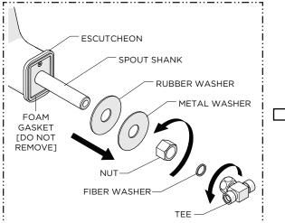
Remove the TEE, NUT and LOWER DECK WASHERS from the SPOUT SHANK.
