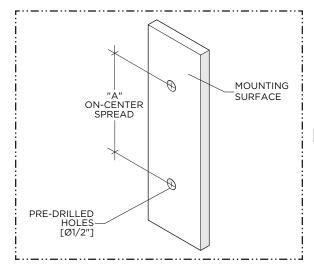
1. Drill two 1/2" diameter holes on the mounting surface at the required on-center spread (DIM A).
