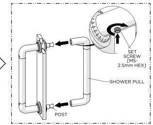
Slide the PULL onto the POSTS until it contacts the ESCUTCHEONS then thread and securely tighten the SET SCREWS.
