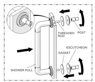
3. Slide the ESCUTCHEONS onto the THREADED RODS then thread and securely tighten the POSTS.
