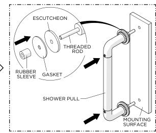
Pre-assemble the ESCUTCHEONS and RUBBER SLEEVES onto the THREADED RODS on the PULL then insert the RUBBER SLEEVES into the predrilled holes.
