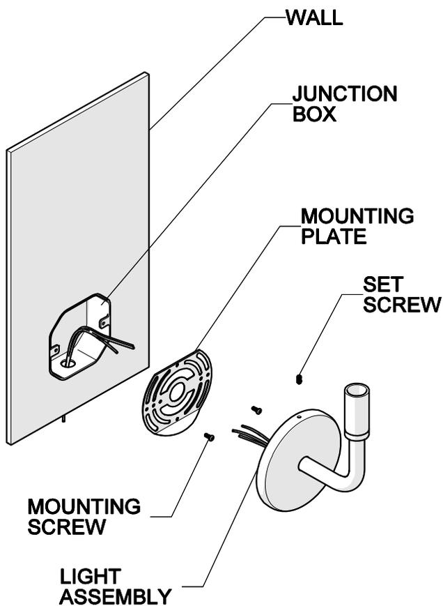
These guidelines have been prepared for the professional contractor to aid in the installation of: FLYTE, LUDLOW, & ROADSTER WALL MOUNTED SINGLE ARM SCONCE (STYLE#S FLLT01 [FLO1LT], LDLT01 [LD01LT], RDLT01 [RD01LT])
