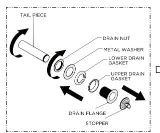
Remove the STOPPER, UPPER and LOWER DRAIN GASKETS, WASHERS, NUT and TAILPIECE from the DRAIN FLANGE.
