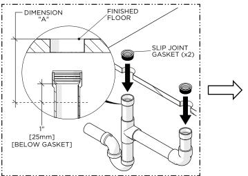
Insert the SLIP JOINT GASKETS (x2) into the HUBS then measure from the finished floor to 1" [25mm] below the bottom of the GASKETS.
