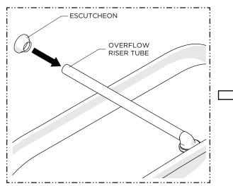
Slide the ESCUTCHEON onto the OVERFLOW RISER TUBE.
