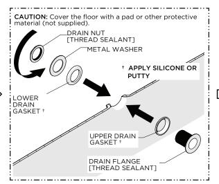
With the BATHTUB on its side, apply a generous bead of silicone or putty to the UPPER and LOWER GASKETS and set the FLANGE then thread and securely tighten the NUT onto the FLANGE.
