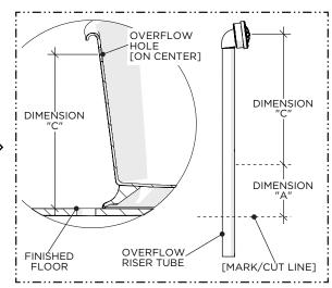
Measure (DIMENSION "C") from the center of the OVERFLOW HOLE to the finished floor then, using the previous DIMENSION "A", mark and cut the OVERFLOW RISER TUBE.
