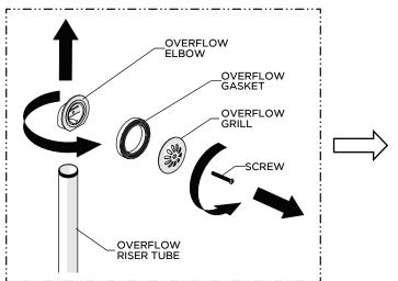
Unthread and remove the SCREW, OVERFLOW GRILL, OVERFLOW GASKET, COLLAR, and ORING. Remove OVERFLOW RISER PIPE from OVERFLOW ELBOW.
