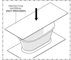
17. Cover the BATHTUB surface with a liner or other protective material (not supplied) until construction is completed.
