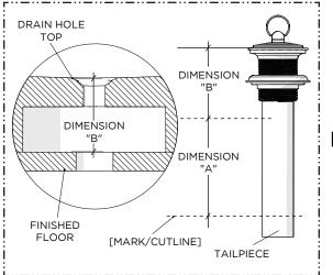
Measure (DIMENSION "B") from the top of the DRAIN HOLE to the finished floor then, using the previous DIMENSION "A", mark and cut the DRAIN TAILPIECE.
