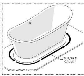
15. Run a bead of tub and tile caulk around the bottom edge of the BATHTUB where it meets the finished floor and wipe away any excess caulk with a wet paper towel.
