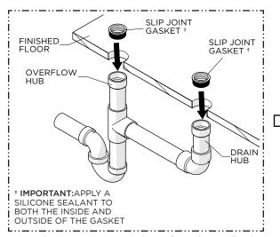
Apply a generous coating of a clear adhesive silicone sealant to both the inside and outside of the SLIP JOINT GASKETS and insert the GASKETS into the DRAIN HUBS.
